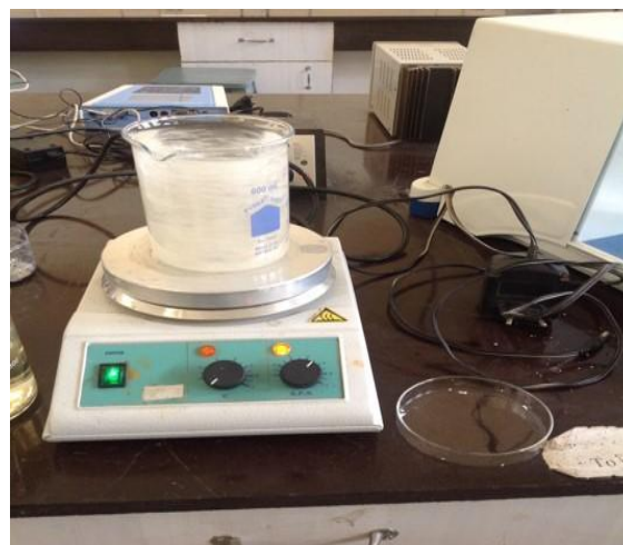
Figure 2(b): PEP being used to treat the water sample with the aid of a magnetic stirrer
