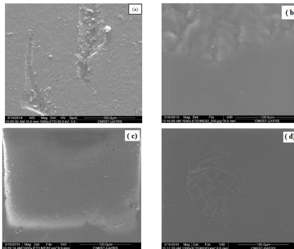
**Figure 12:** SEM images for the four samples after the immersion for 48 hours in 3% NaCl solution.
