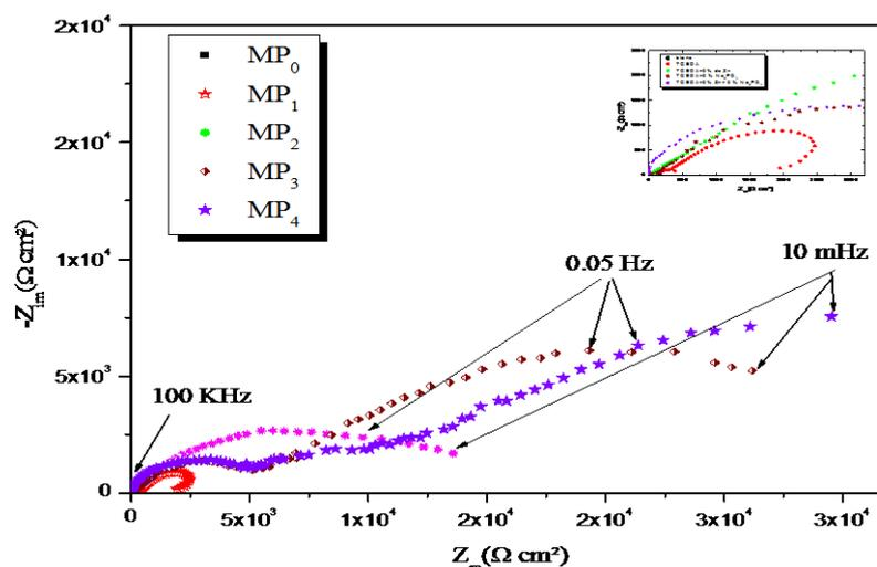
**Figure 10:** Electrochemical impedance diagrams with open circuit after 30 min of immersion for carbon steel in 3% NaCl in the presence of matrices (MP<sub>0</sub>, MP<sub>1</sub>, MP<sub>2</sub>, MP<sub>3</sub> and MP<sub>4</sub>) (Transition Method) at 298 K.
