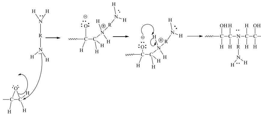
**Figure 3:** The proposed mechanism for the reaction of an epoxy resin and a primary diamine as a hardener.
