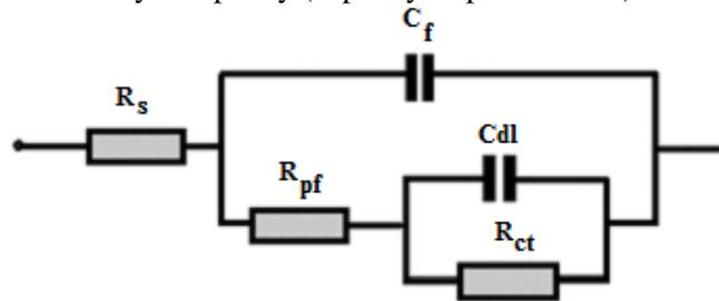
**Figure 11:** Equivalent circuit provided for the adjustment of dies for spectra of impedance obtained in the presence of different matrices for carbon steel in 3% NaCl.
