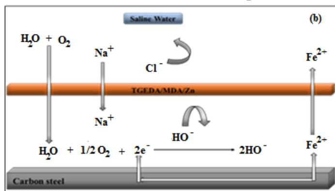
Figure 8: mechanism of formation of the passivation coating at the interface between the metal substrate and the film after the immersion in 3% NaCl.
