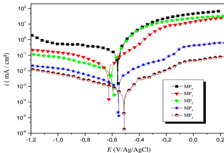
**Figure 6:** Carbon steel polarization curves in 3% NaCl at different matrices after 30 min immersion at 298 K.
