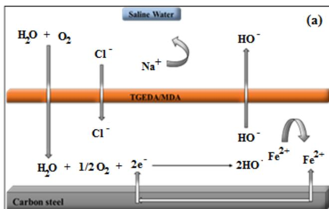
Figure 7: Mechanism proposed for the protective matrix  $MP_1$  (TGEDA/MDA) between the metal substrate and the film after the immersion in 3% NaCl.
