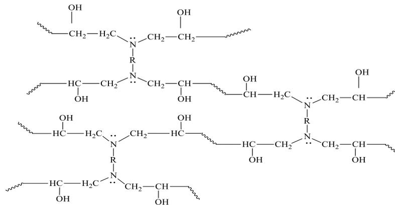
**Figure 4:** Structure of idealized epoxy resins and primary diamines as hardening agent.
