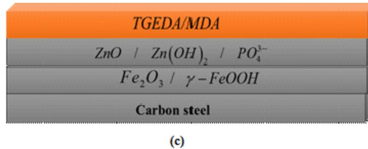
**Figure 9:** Diagram of the passivation coating induced by the presence of zinc phosphate pigments [30].
