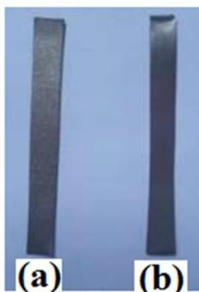
**Figure 1:** Titanium surface; (a) before preparation; (b) after preparation.
