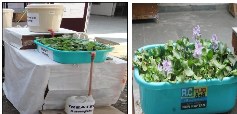
Figure 2 and 3: Constructed Wetland design and set up using E. crassipes
