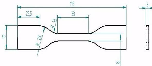
**Figure 5:** Tensile Test specimen (ASTM D – 638)
