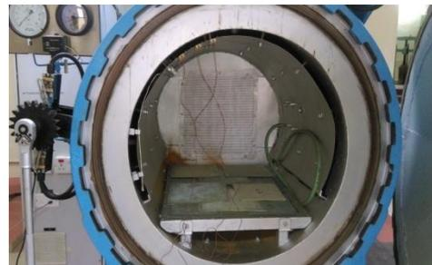
**Figure 4:** Laminates Placed Inside Autoclave Machine
