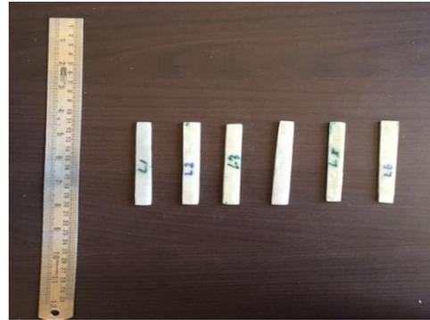
Figure 13: Flexural Test Specimen for testing
