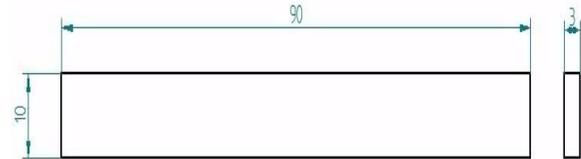
**Figure 6:** Flexural Test specimen (ASTM D – 790)
