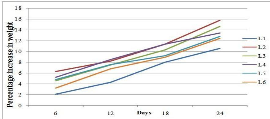
Figure 24: Water Absorption Test Results for normal water
