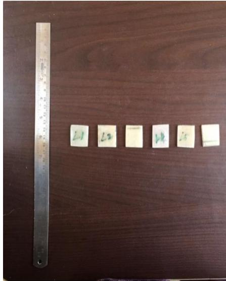
**Figure 16:** Water Absorption Testing Specimen
