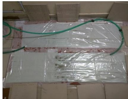
**Figure 2:** Laminates laid-up on the mat
