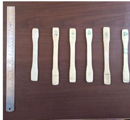
Figure 11: Tensile test Specimen before for testing
