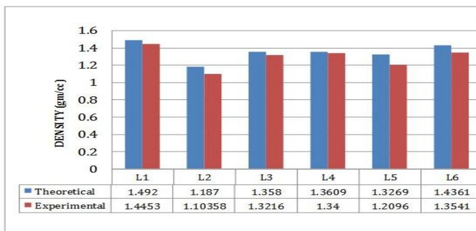
**Figure 18:** Theoretical and Experimental Density of Laminates
