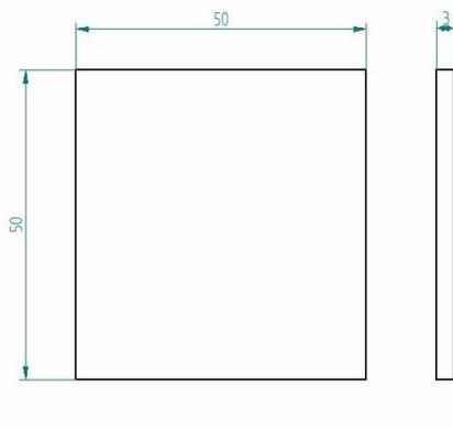
**Figure 8:** Hardness Test specimen (ASTM E - 384)
