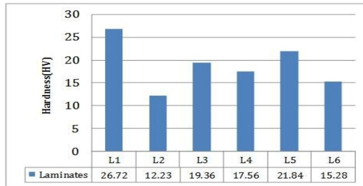
Figure 25: Hardness Test results of Laminates
