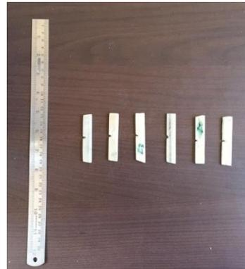
Figure 15: Flexural Test Specimen for testing
