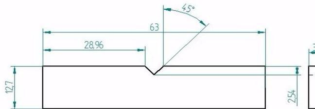
**Figure 7:** Impact Test specimen (ASTM D – 256)
