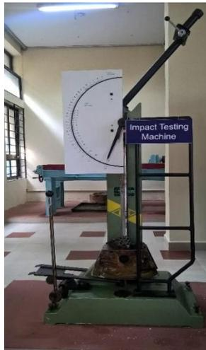
Figure 14: Impact Testing Machine
