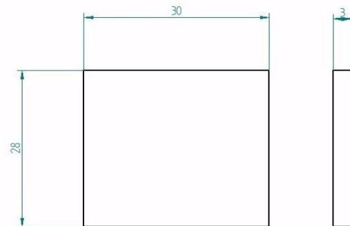
**Figure 9:** Water absorption test specimen (ASTM D - 570)
