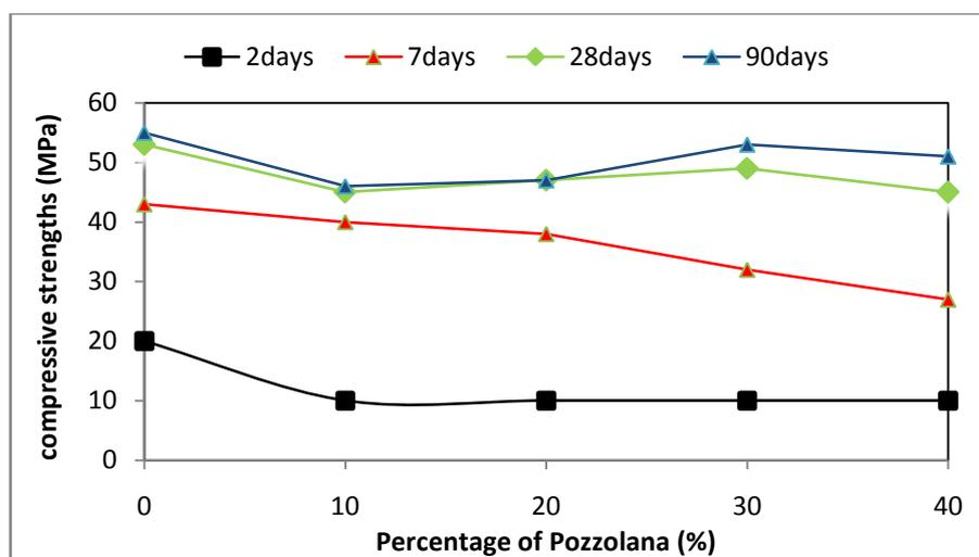
Figure 1: Effect of the pozzolan on the CPA compressive strength
