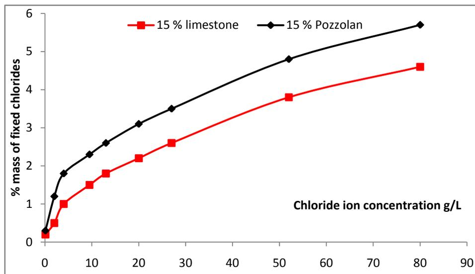
**Figure 4:** Percentage mass of fixed chloride on concrete matrix with 15% limestone and 30% pozzolan in function the concentration of Cl<sup>-</sup>
