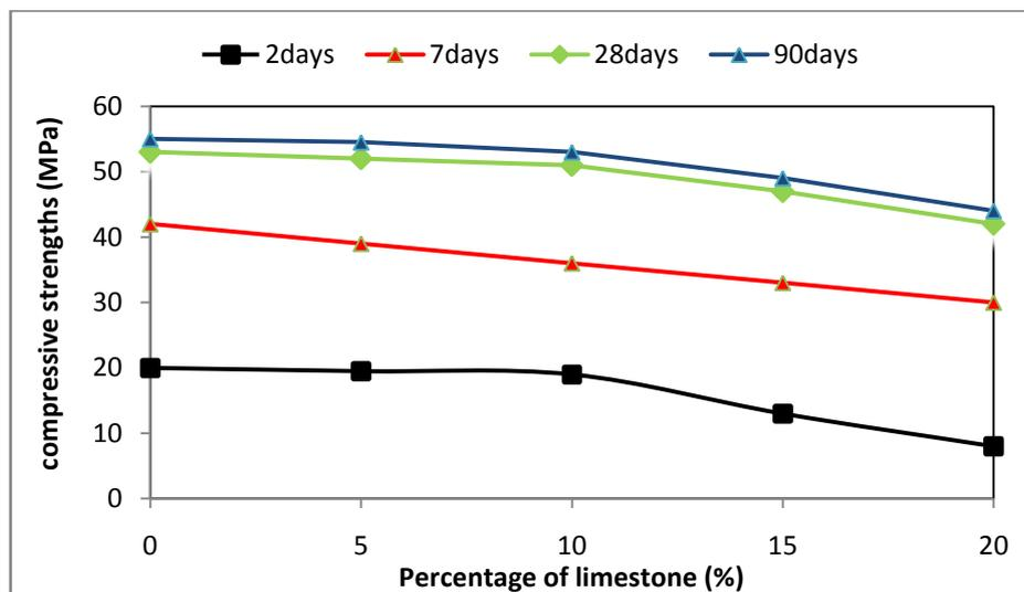
**Figure 2:** Limestone effect on the compressive strength of the CPA cement
