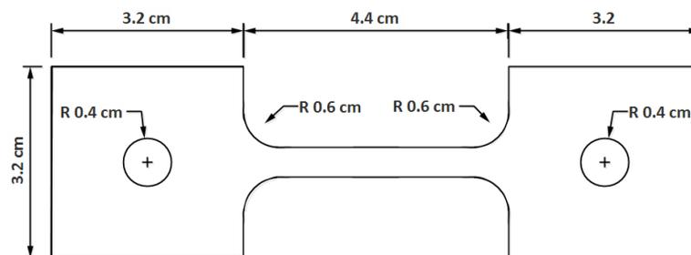
**Figure 1:** Schematic diagram of steel sample with dimensions.
