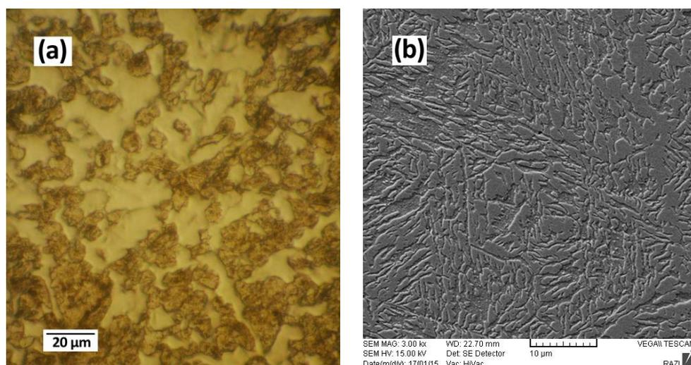
**Figure 3:** Optical and SEM micrographs for intercritical annealed specimen at 740 °C.
