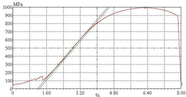
**Figure 10:** Engineering stress-engineering strain curves of intercritical annealed specimen 860 °C.
