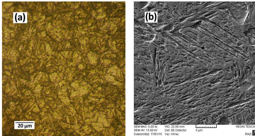
**Figure 9:** Optical and SEM micrographs for intercritical annealed specimen at 860 °C.
