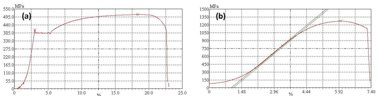
**Figure 5:** Engineering stress-engineering strain curves of (a) normalized specimen and (b) intercritical annealed sample at 740 °C.
