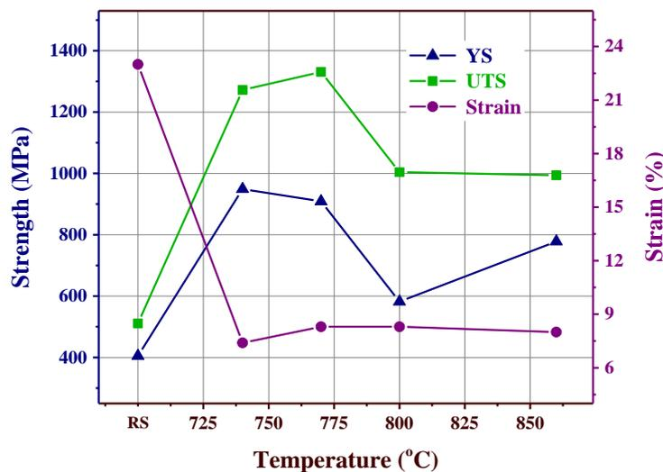
**Figure 4:** Variation of yield strength (YS), ultimate tensile strength (UTS) and strain versus intercritical annealing temperature.
