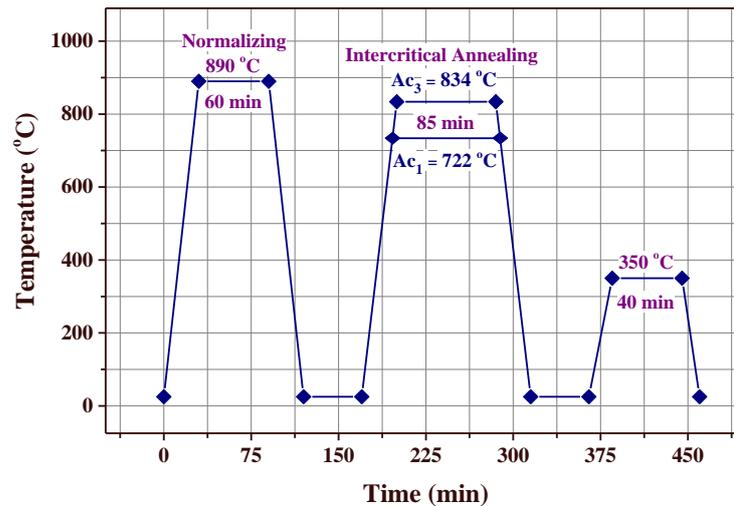
**Figure 2:** Schematic illustration of heat treatment cycle used in this study.
