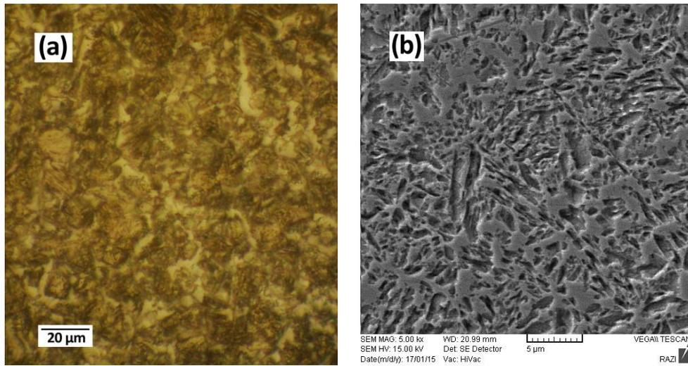
**Figure 8:** Optical and SEM micrographs for intercritical annealed specimen at 800 °C.
