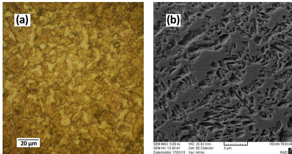
Figure 6: Optical and SEM micrographs for intercritical annealed specimen at 770 °C.
