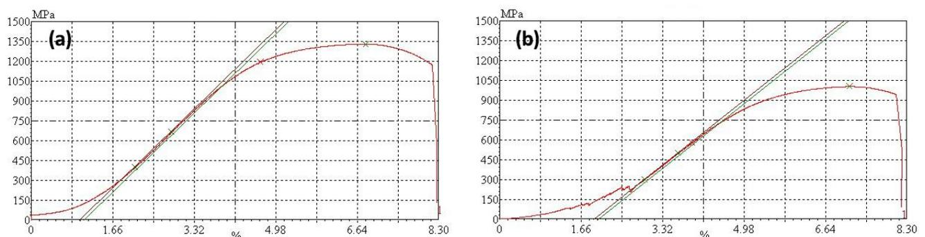
Figure 7: Engineering stress-engineering strain curves of intercritical annealed specimens at (a) 770 and (b) 800 °C.
