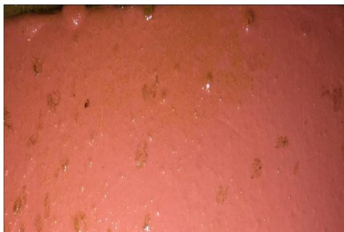
**Figure 7:** Fouling in the form of islands on antifouling paints with 6 percent Zineb and Ziram after 59 days of immersion in sea water
