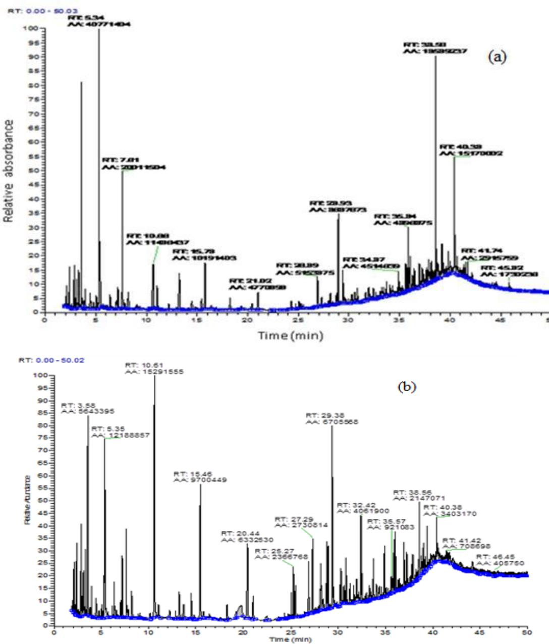
**Figure 7:** Chromatogram of bio-oil (a) 500/200 at 500 °C, (b) 315HD at 450°C
