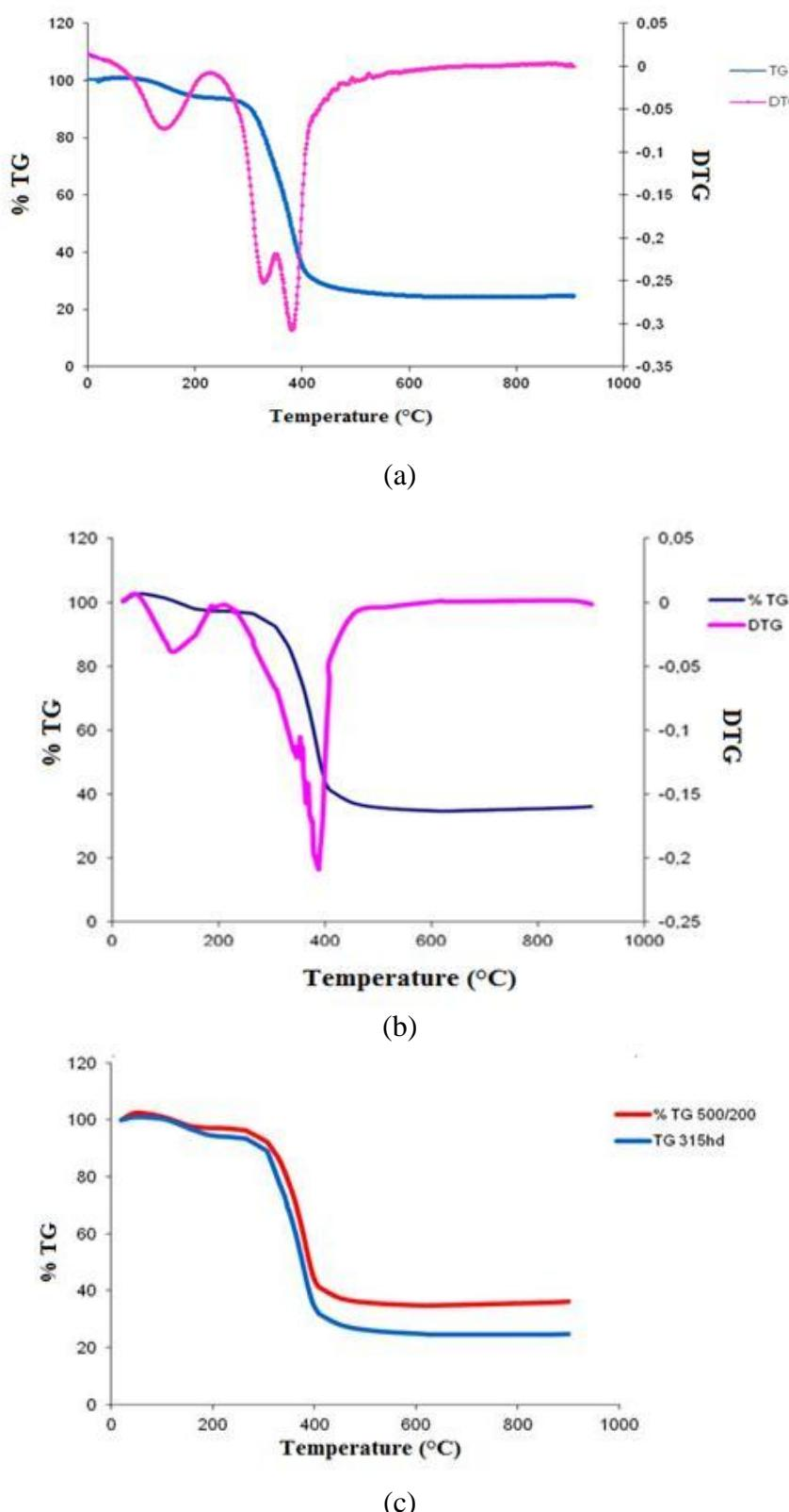
**Figure 2:** TGA curves with temperature increase velocity of 100°C/min, (a) 315HD, (b) 500/200, (c) comparison of ATG of 315HD and 500/200
