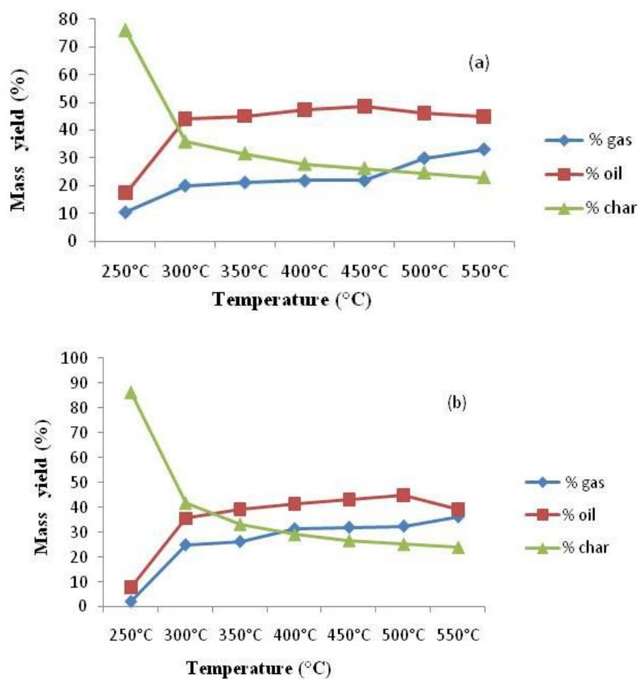
**Figure 3:** Influence of the temperature on the yield of the products of pyrolysis (a) 315HD, (b) 500/200
