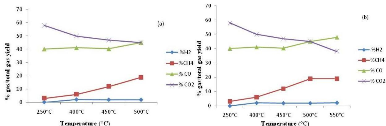
**Figure 4:** Influence of the temperature on the gases production from wood pyrolysis (a) 315HD, (b) 500/200
