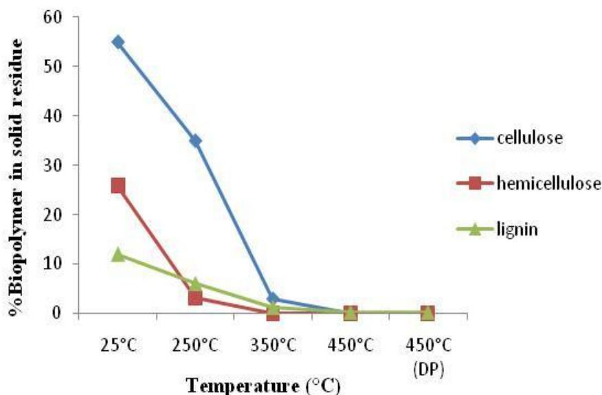
**Figure 8:** Influence of the staged pyrolysis on the macro-components content in the solid residue of the biomass 315HD
