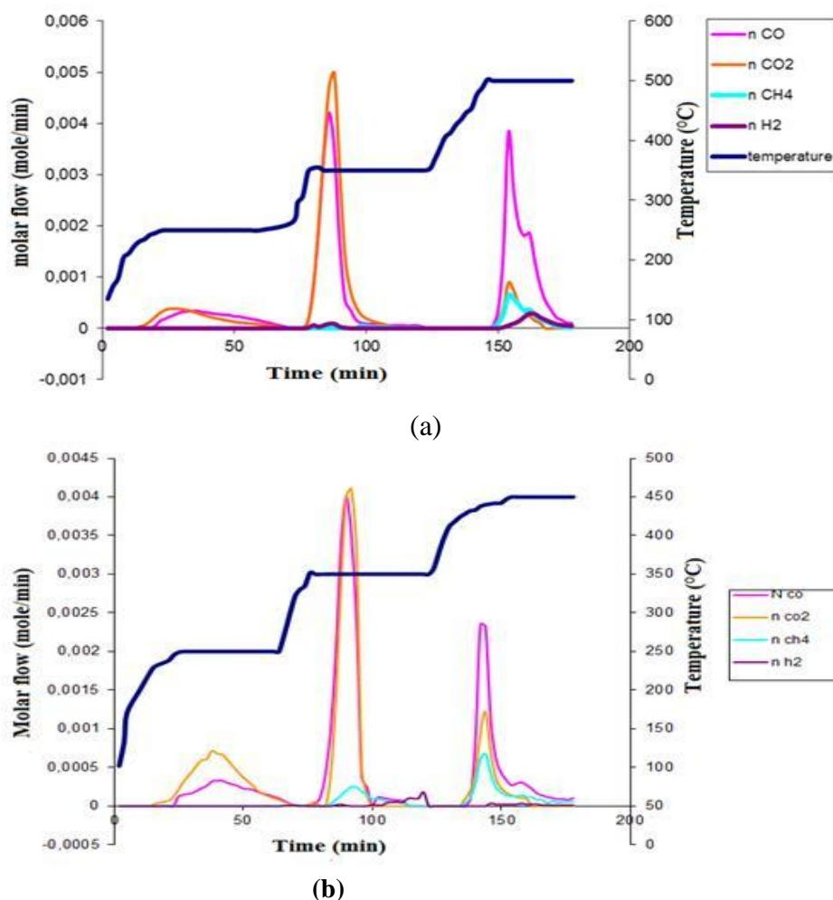
**Figure 9:** Production of gases during the staged pyrolysis of the biomasses (a) 500/200,(b) 315HD
