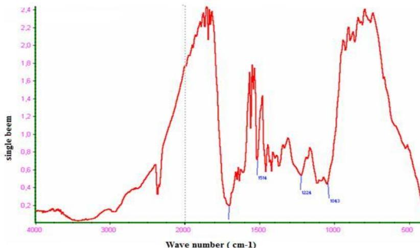
**Figure 6:** IR spectrum of the bio-oil obtained by pyrolysis of 315HD at  $450^\circ\text{C}$
