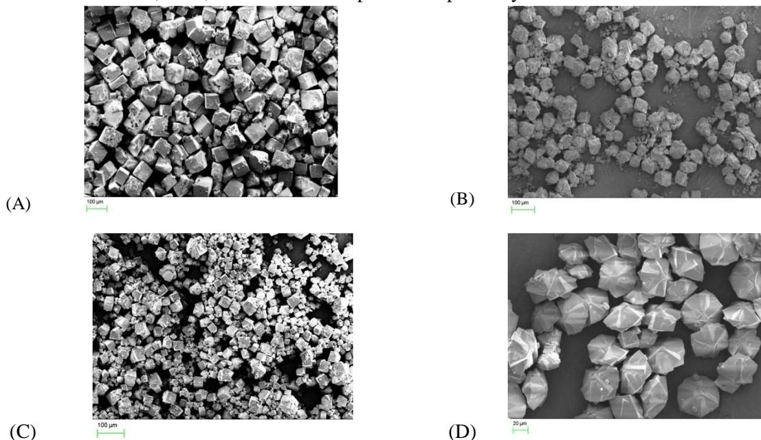
**Figure 2:** SEM images of samples synthesized using various templates (A) DEA (B) TEA (C) TEAOH (D) Morpholine
