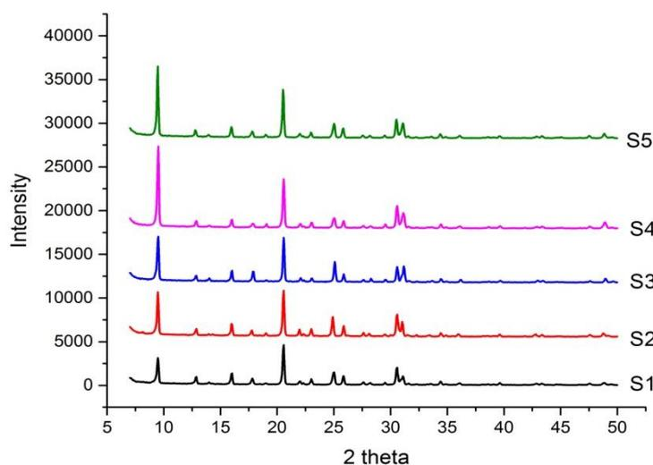
**Figure 1:** XRD patterns of as synthesized SAPO-34
