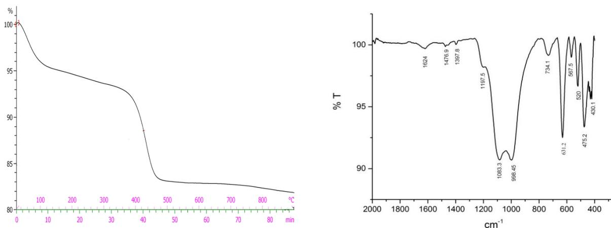
**Figure 5:** FTIR spectra of SAPO 34 sample synthesized with DEA and colloidal silica
