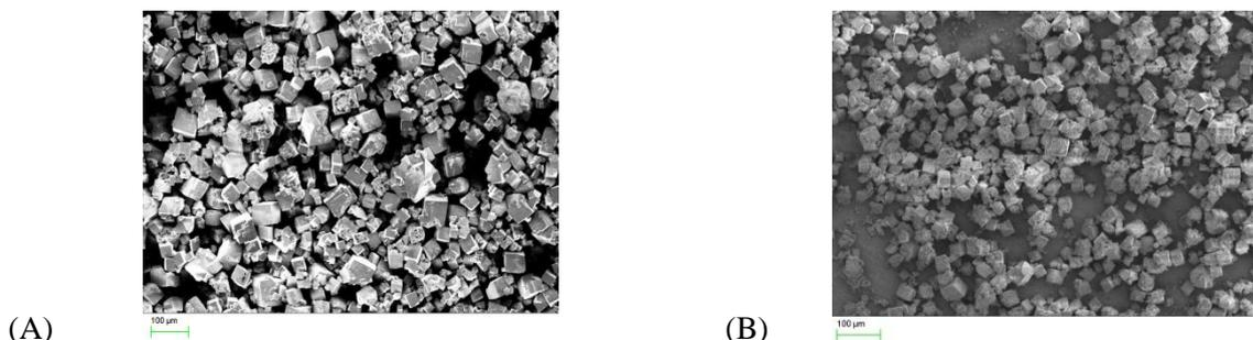
**Figure 3:** SEM images of samples synthesized using DEA as template with different silicon sources (A) Fumed silica (B) Colloidal silica
