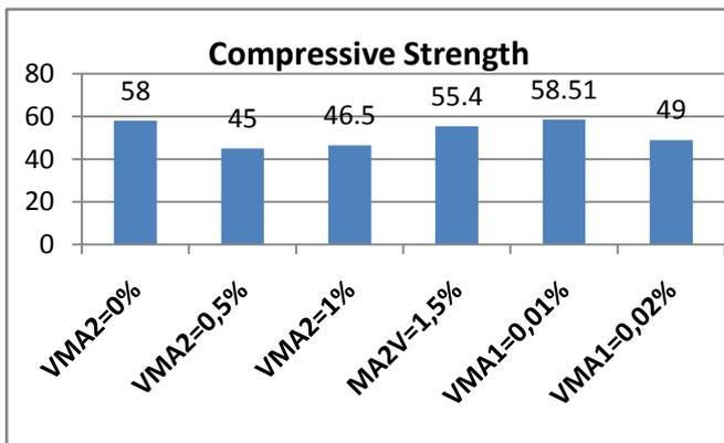
Figure 8: Compressive Strength for SP=1.8%
