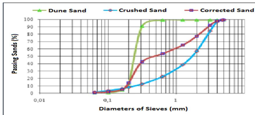
Figure 1: Grading curves of used sands
