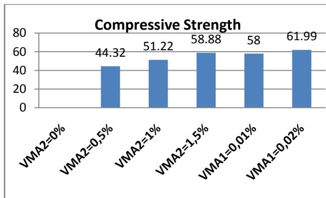
Figure 14: Compressive Strength for SP=2.4%
