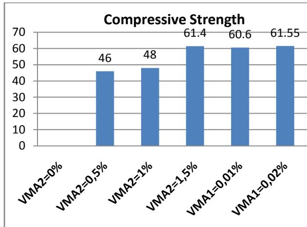
Figure 12: Compressive Strength for SP=2.2%
