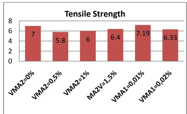
Figure 9: Tensile Strength for SP=1.8%
