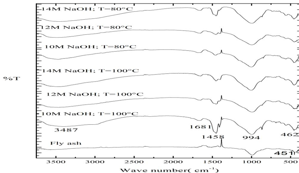
**Figure5:** infrared analysis of fly ash and alkali activated fly ash at different NaOH concentrations under two curing conditions (80 and 100°C)
