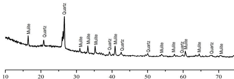
**Figure 2:** XRD profile of fly ash
