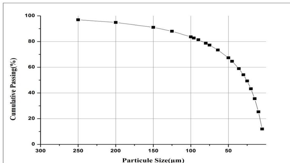
**Figure1:** Particle size distribution of fly ash
