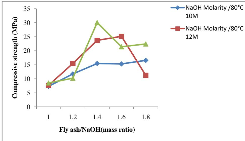
**Figure 3:** Compressive strength of alkali-activated fly ash at 80°C
