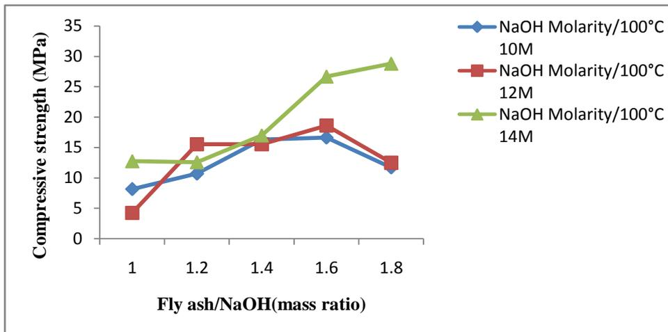
**Figure 4:** Compressive strength of alkali-activated fly ash at 100°C
