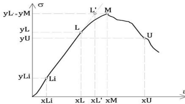
**Figure9:** Identification of the characteristics points in stress-strain diagram
