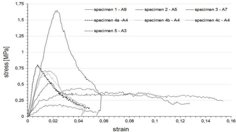
**Figure 12:** Stress-strain diagram of specimens of period VII and VI A
