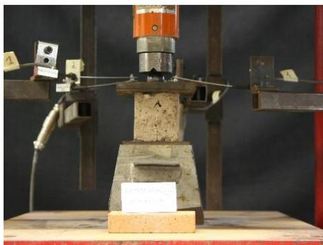
**Figure7:** Compression test apparatus
