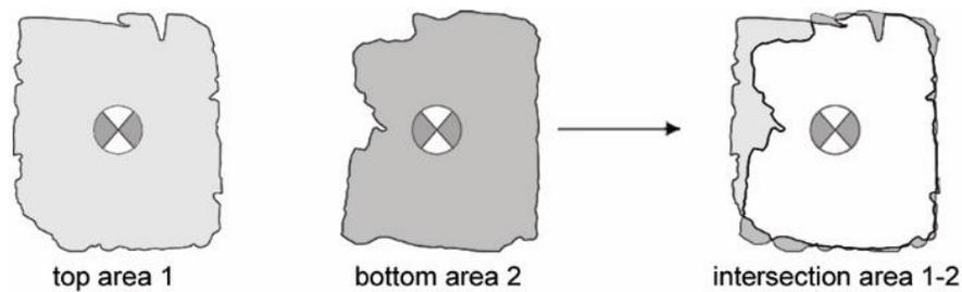
**Figure6:** Identification of the actual effective resistant surface in the 9a specimens.
