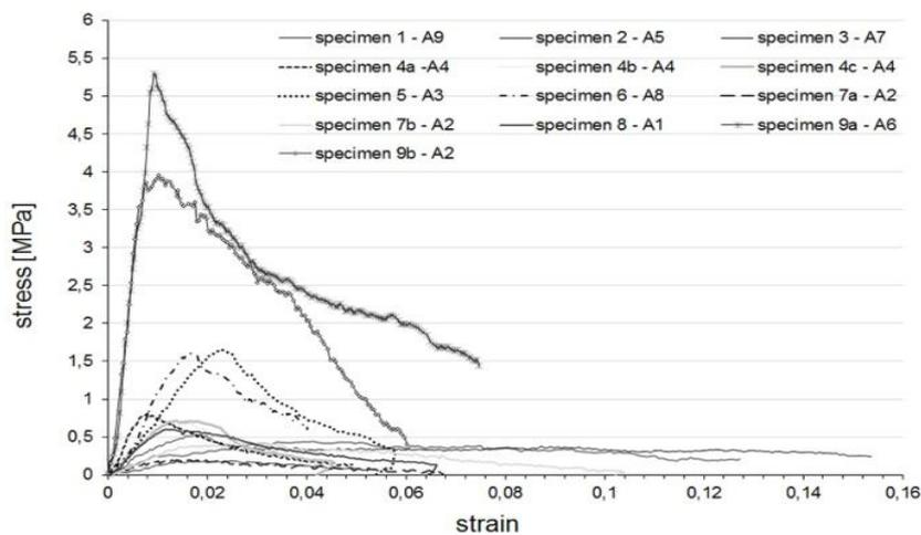
**Figure10:** Stress-Strain diagrams for all the tested specimens
