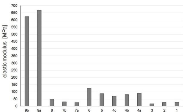
**Figure 13:** Elastic modulus of all specimens
