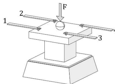
**Figure8:** Compression test apparatus, schema
