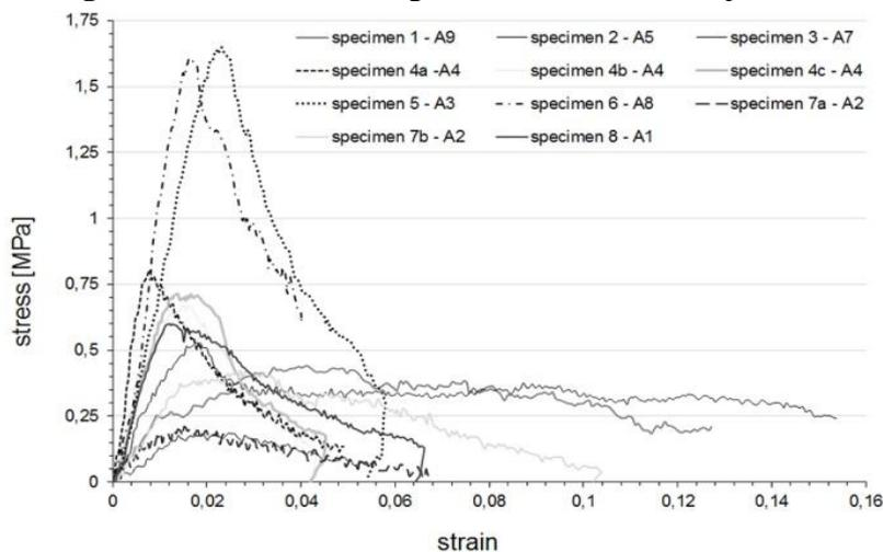
**Figure 11:** Stress-strain diagrams for all specimens without 9a and 9b specimens that exhibited much greater mechanical properties.
