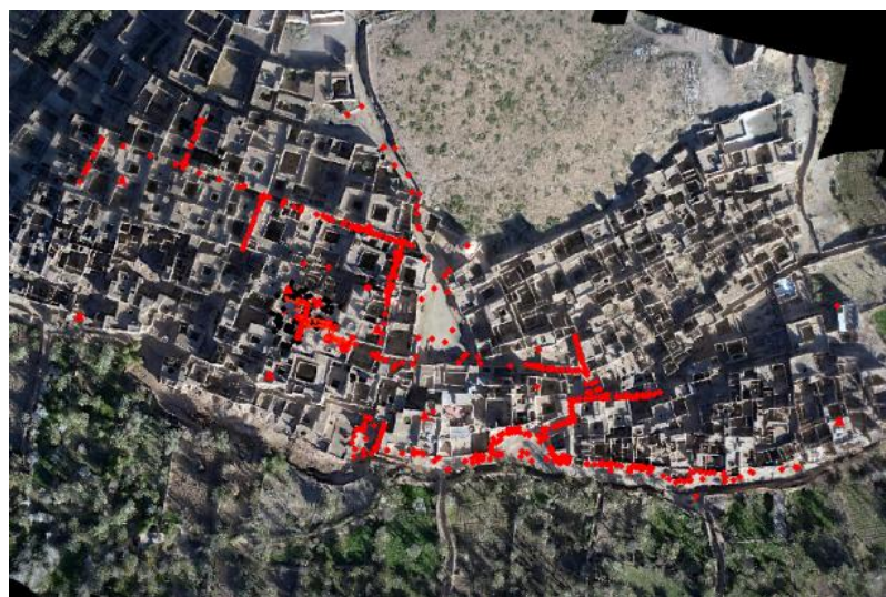
Figure 4: Aerial view from the Ksar of Tamnougalt, additional terrestrial measurement for ground control points.
