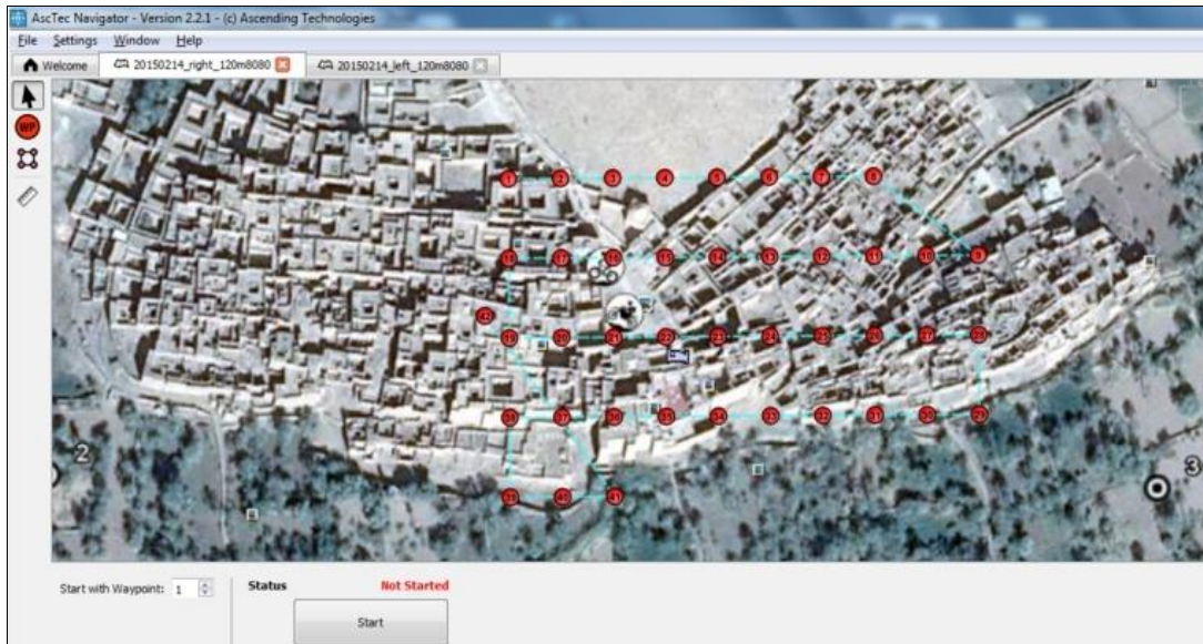
Figure 3: Flight altitude of the unmanned aerial vehicle (UAV): 120m, 4 short flights with longitudinal and cross imbrications of 80%, ground resolution 3cm, marked air track of the second flight (red dots).
