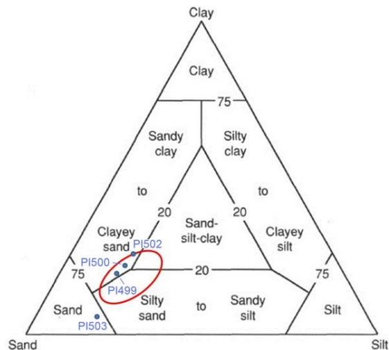
**Figure 5:** Shepard diagram with the points of the rammed earth masonries of wall D (PI499, PI500) and wall E (PI502). In red the optimal granulometric composition” reported by CRA Terre for rammed earth
