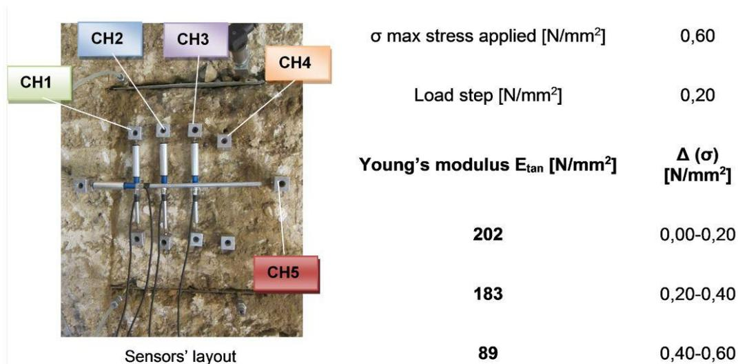
**Figure 8:** Flat jack test on the rammed earth of the wall D, in the northern side.
