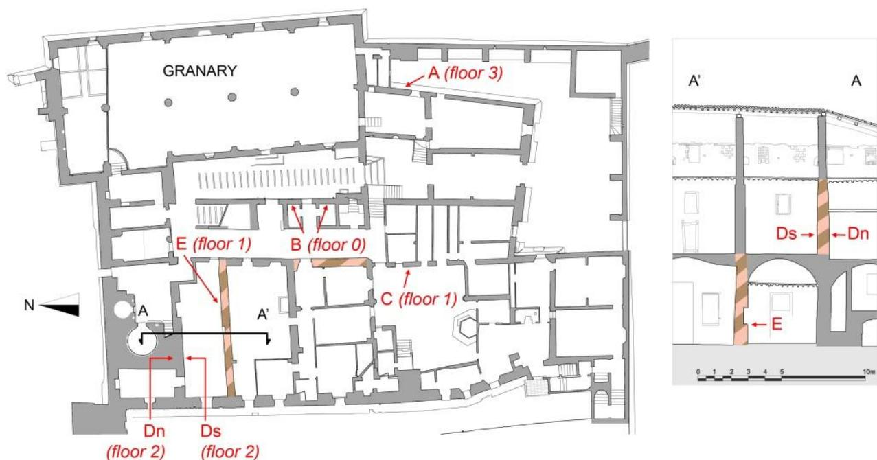
**Figure 2:** Grange of Cuna - plant of the first floor and A-A' section, with indication of the sampling points. A, B, C: brick masonries with earthen bedding mortar; D, E: rammed earth masonries (Ds: wall D, southern side; Dn: wall D, northern side). Pink and brown masonries: rammed earth masonries alternating with brick masonries with lime bedding mortar.
