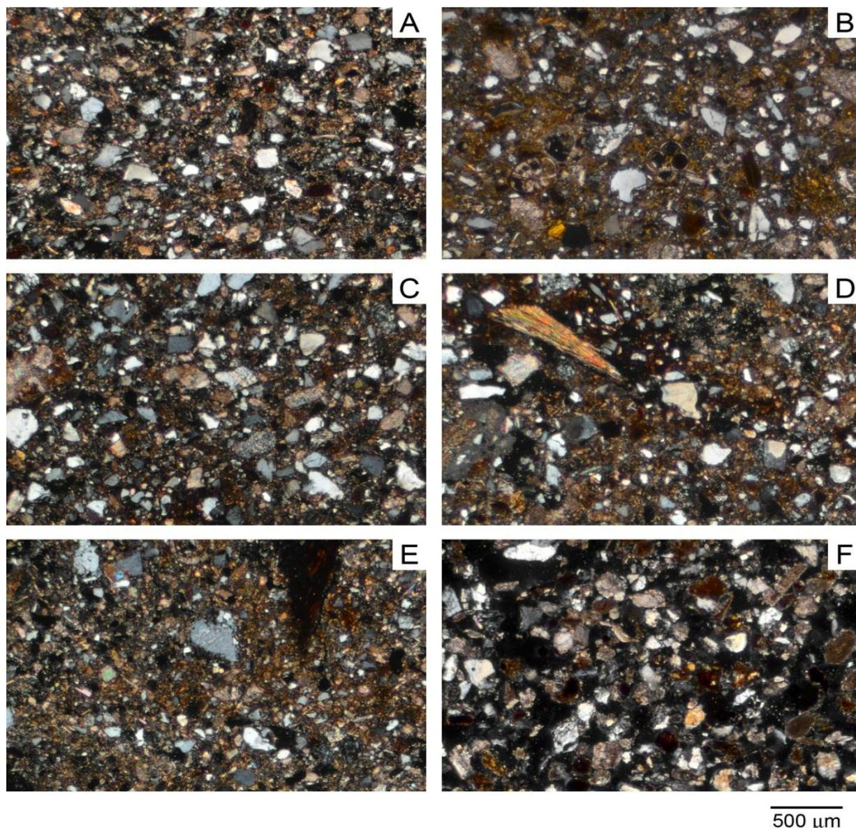
**Figure 6:** Polarized light microscopy images in thin section of a selection of the samples of earthy materials analysed (all obtained under crossed polarizers). Earthen bedding mortar samples: **A** - PI207 (wall A); **B** - PI236 (wall B); **C** - PI503 (wall C). Samples from the rammed earth masonries: **D** - PI499 (wall D, southern side); **E** - PI502 (wall E). **F** - Sandy material collected from the Arbia Stream bank (sample PI231).
