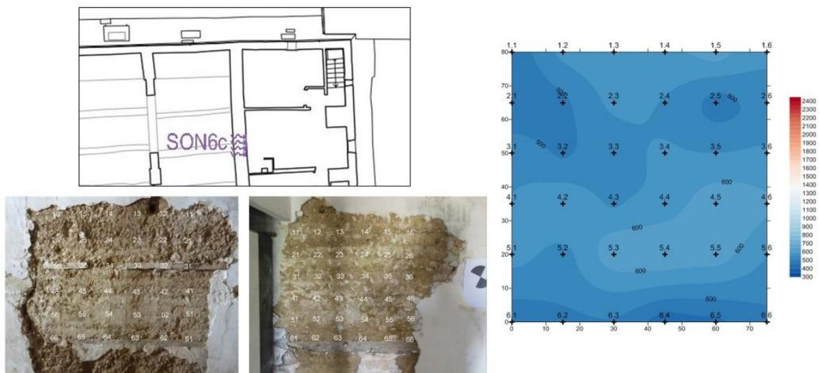
**Figure 10:** Sonic test on the rammed earth of the masonry D with the graphical representation of the velocity values (m/s).
