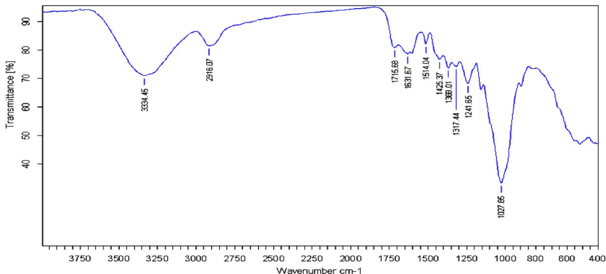
**Fig.1.** Spectroscopy infra red of corn cob powder calcined (CCPC).
