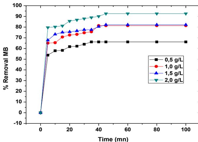
**Fig.4.** Effect of adsorbent amounts on dye removal of MB. Interval of adsorbent dose (0.5-2 g/L), Initial dye concentration 100 mg/L, V=200 mL pH=6.8, T= 20 °C and agitation time 100 min.
