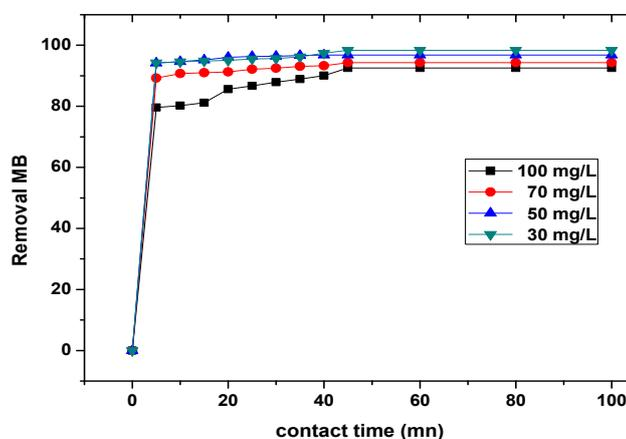
Fig.3. Effect of contact time and dye concentration adsorbent. Interval of initial concentration (30 to 100 mg/L), adsorbent dose: W= 0.4 g, V= 200 mL, pH=6.8, T= 20 °C and agitation time 100 min.
