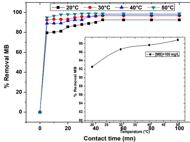
Fig.6. Effect of temperature on the adsorption kinetics of MB onto CCPC.
