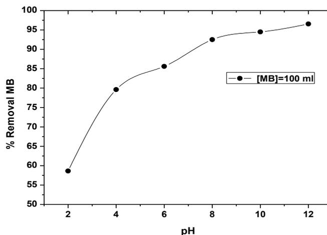
**Fig.5.** Effect of pH on removal of MB onto CCPC. Interval of pH (2-12), Initial dye concentration 100 mg/L. Adsorbent dose: W= 0.4 mg, V=200 mL, T= 20 °C and agitation time 100 min.
