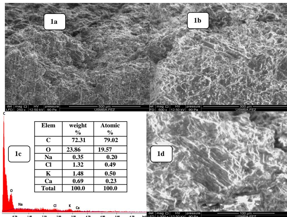
Figure 2. SEM Microscopy coupled by EDX, for CCPC (1a, 1b, 1c, 1d)
