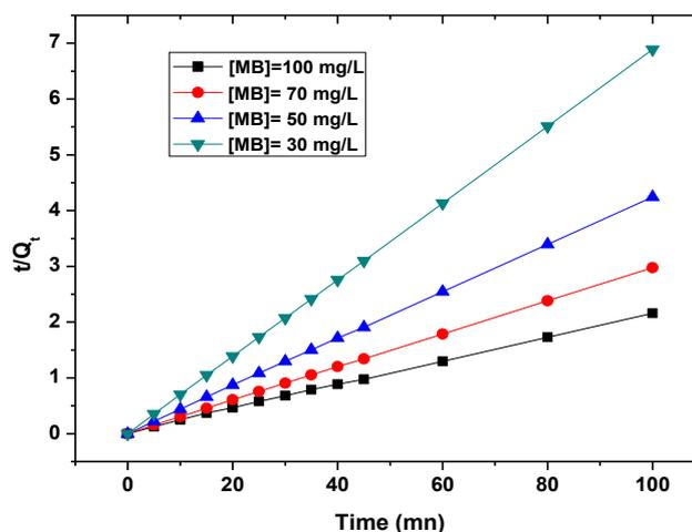
**Figure 12:** Model of the pseudo-second-order for the adsorption of the methylene blue on the adsorbent CCPC
