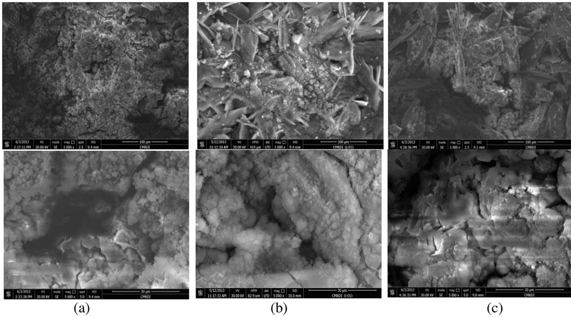
**Figure 11:** SEM morphology for (a) additive-free (b) PEG-additive (c) SLS-additive coatings after corrosion testing in the SBF solution.
