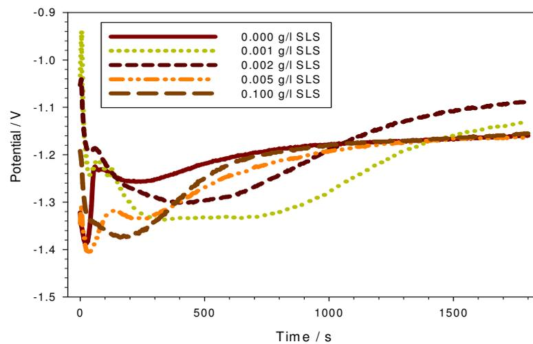
**Figure 3:** Potential-time curve of FHA coatings in the SBF solution containing different concentrations of SLS compound
