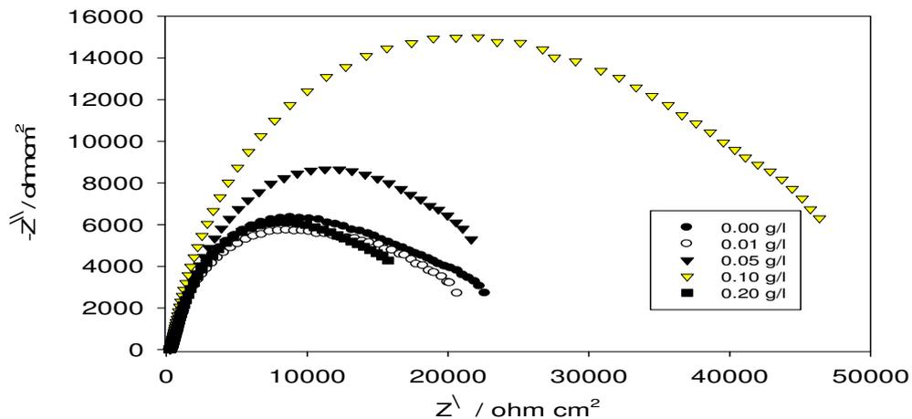
**Figure 4:** Nyquist plots of FHA coatings in the SBF solution containing different concentrations of PEG compound
