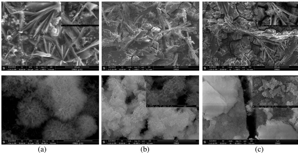
**Figure 10:** SEM morphology for (a) additive-free (b) PEG-additive (c) SLS-additive coatings before corrosion testing in the SBF solution.
