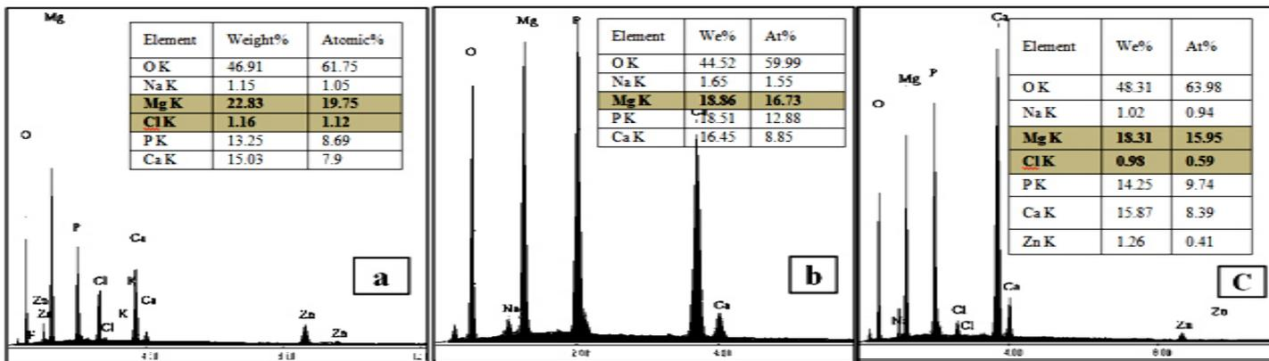
**Figure 13:** EDS analysis of FHA coating in the absence (a) and in the presence of PEG (b) and SLS (c) after corrosion testing in the SBF solution
