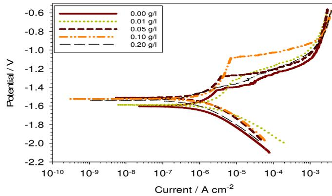
**Figure 8:** Potentiodynamic curves of FHA coats in the SBF solution containing different concentrations of PEG compound
