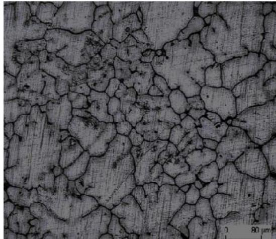
**Figure 1.** Microstructure of the alloy specimen, X= 100
