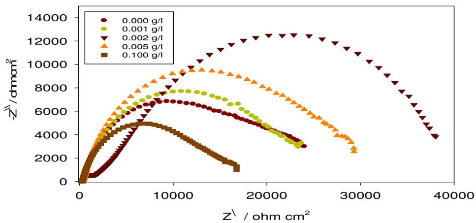
**Figure 6:** Nyquist plots of FHA coatings in the SBF solution containing different concentrations of SLS compound
