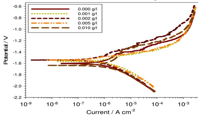
**Figure 9:** Potentiodynamic curves of FHA coats in the SBF solution containing different concentrations of SLS compound
