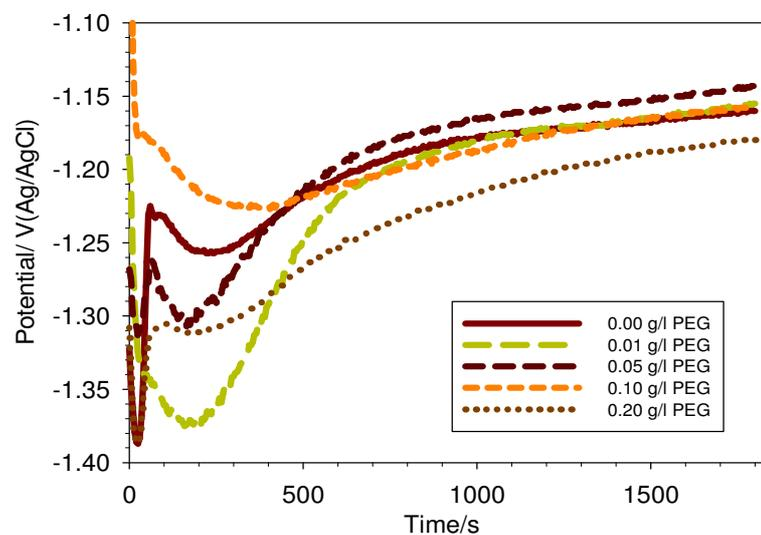
**Figure 2:** Potential-time curve of FHA coatings in the SBF solution containing different concentrations of PEG compound
