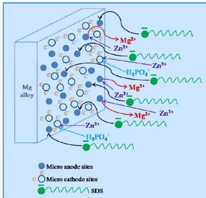
**Figure 14:** Schematic illustration for charged particles molecules effect on coating deposition on the surface of the Mg alloy. *Amini and Sarabi, Appl. Surf. Sci., 257 (2011) 7134 [11]*
