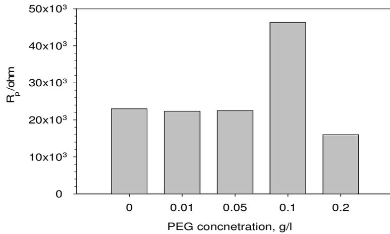
**Figure 5:** Polarization resistance derived from Nyquist plots of FHA coatings in the SBF solution containing different concentrations of PEG compound
