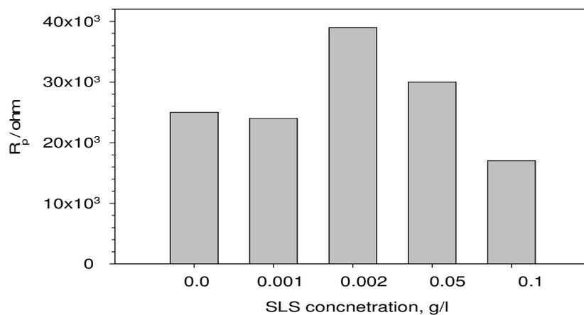
**Figure 7:** Polarization resistance derived from Nyquist plots of FHA coatings in the SBF solution containing different concentrations of SLS compound
