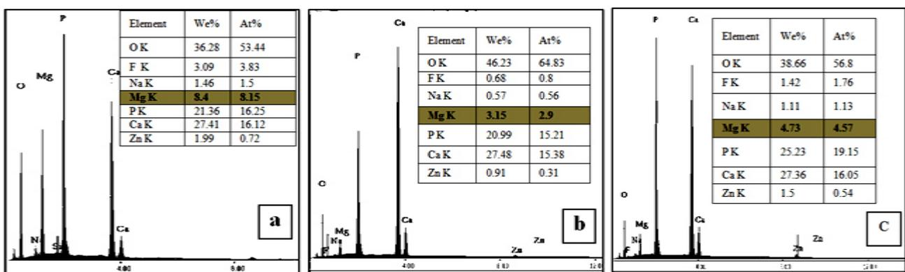
**Figure 12:** EDS analysis of FAH coating in the absence (a) and in the presence of PEG (b) and SLS (c) before corrosion testing in the SBF solution
