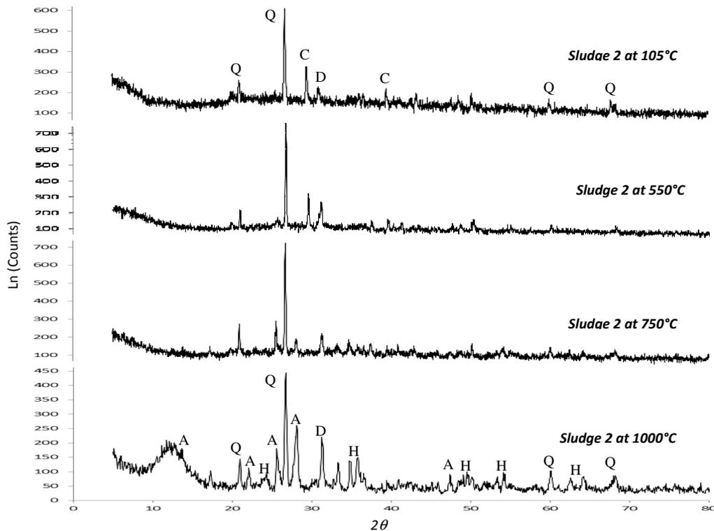
**Figure 6:** XRD spectra of raw sludge 2 and after its heating at different temperatures (A: Albite ; C: Calcite ; D: Dolomite ; H: Hematite ; Q: Quartz).
