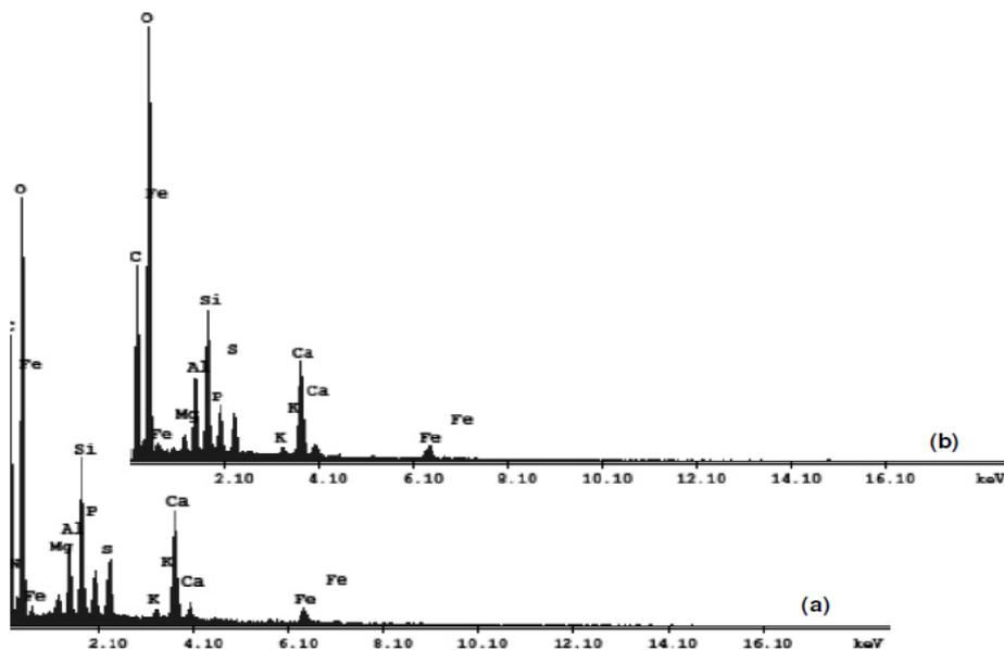
**Figure 12:** Microanalysis done with EDAX for compost samples after 9 months of composting: compost of sludge (a) and compost of the mixture 75% sludge/ 25% sawdust (b).
