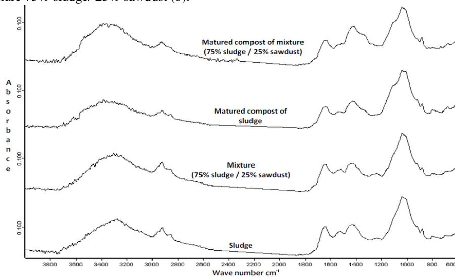
**Figure 13:** ATR-FTIR spectra obtained for, in decreasing order, matured compost of the mixture (sludge/sawdust: 75/25), matured compost of sludge 1, mixture (sludge/sawdust: 75/25) and sludge 1.
