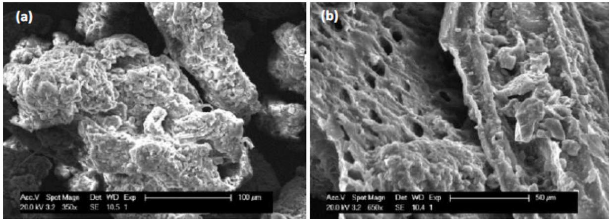
**Figure 11:** SEM Micrographs of compost obtained from sludge 1 (a), and the mixture of 75% sludge and 25% sawdust (b).
