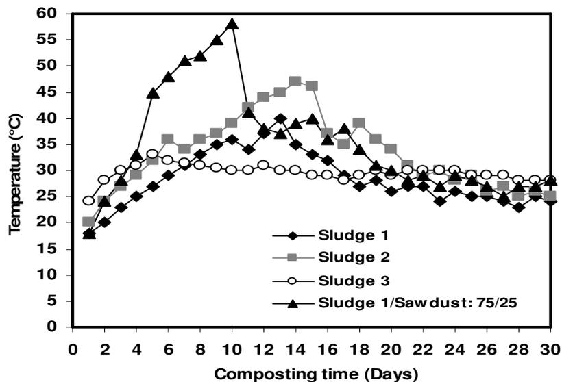
**Figure 7:** Temperature changes during composting process of sludges 1, 2 and 3 and of sludge 1 mixed with sawdust (75/25).
