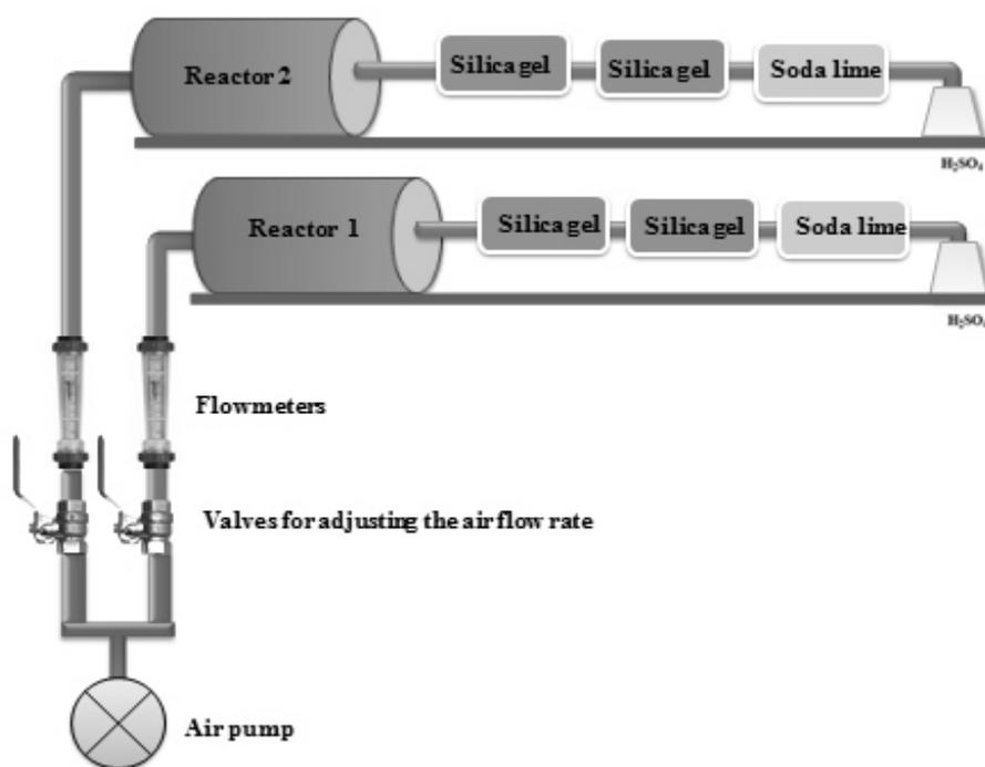
**Figure 1:** Laboratory pilot plant used for composting.
