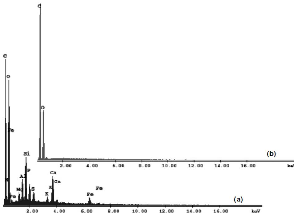
Figure 3: Microanalysis done with EDAX for raw materials: sludge (a) and sawdust (b).
