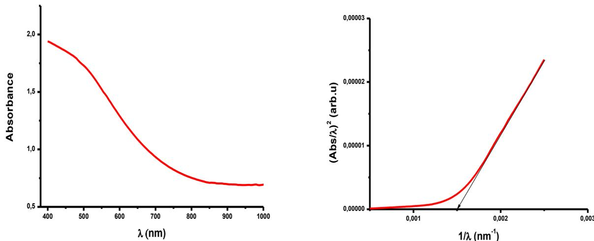
**Figure 3:** Absorbance (a) and ASF plot (b) of CZTS thin film deposited by spin coating
