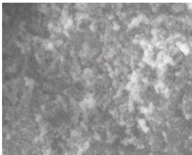
**Figure 2:** Surface morphology of the CZTS thin film
