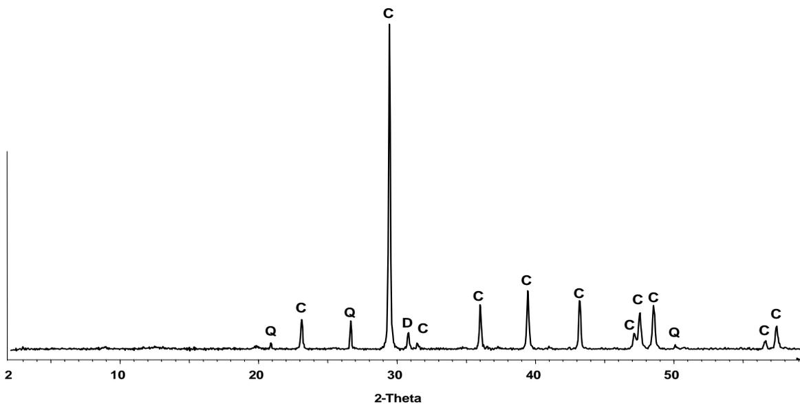
**Figure 4:** XRD Pattern of prehomogenized mixture.
