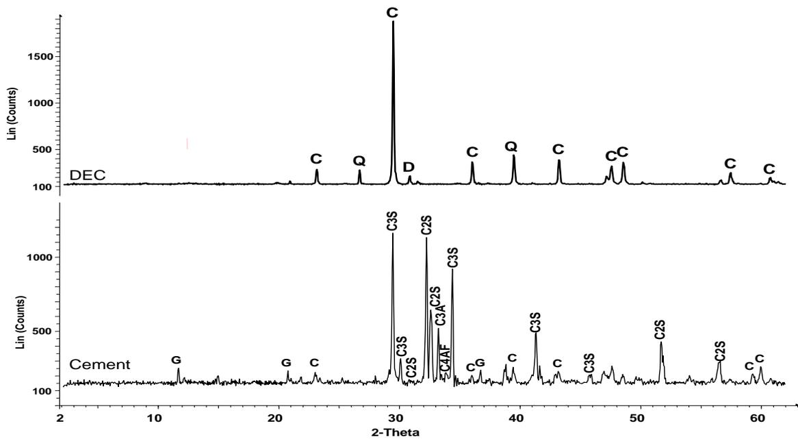
**Figure 5: XRD Pattern of the dust emitted from chimney (DEC), and of the Portland cement.**
