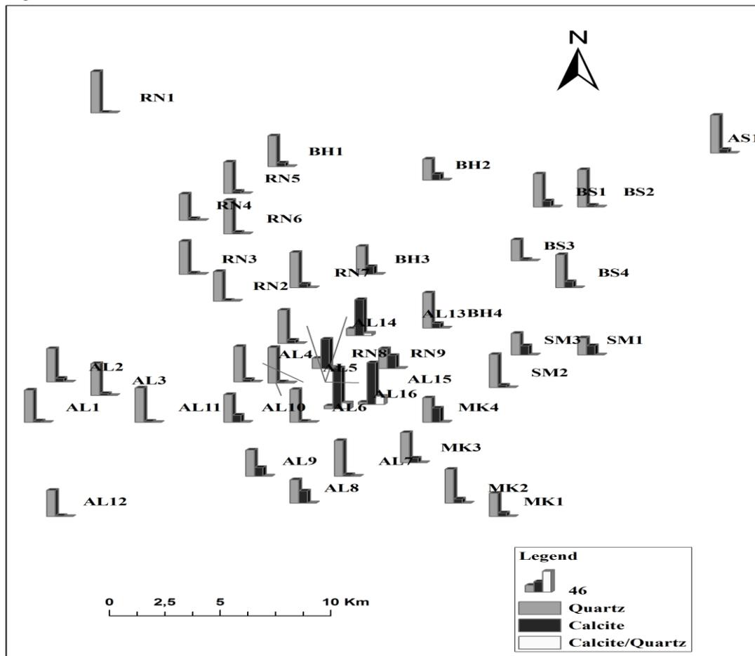
Figure 8: Spatial distribution of calcite, quartz and ratio calcite/quartz.
