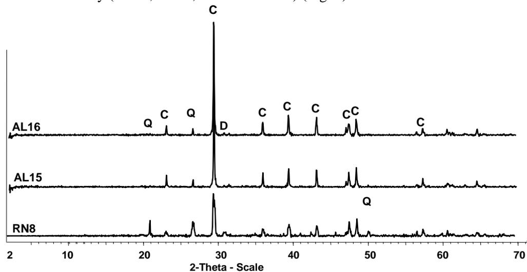
**Figure 6: XRD Pattern of the dusts deposited within the cement factory and its near neighborhoods.**
