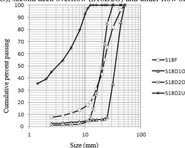
**Figure 1-** curve of graining flows of screen SC18
