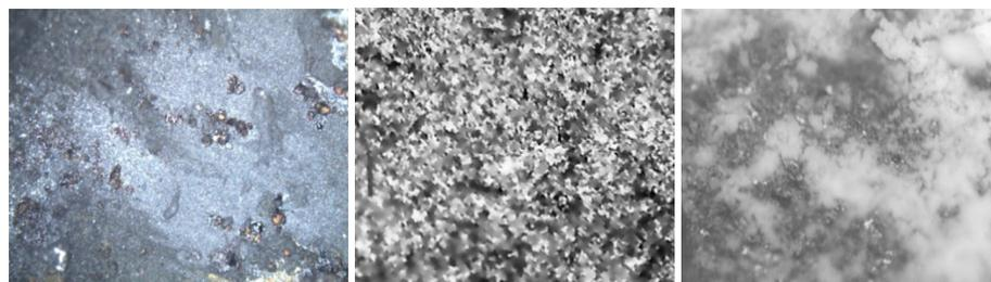
**Figure 6.** Optic picture of Cu–10Ni surface in 0,5M NaCl without 35 ppm of nalco (a) and (b) with 35 ppm.
