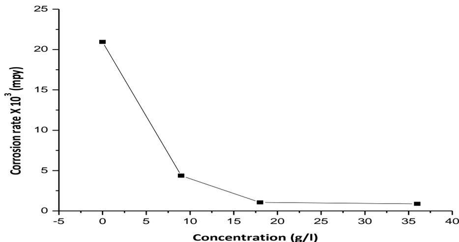
**Figure 2:**Corrosion rate of mild steel at different concentrations of AME in Conc. HCl for 20 min exposure at 25°C.
