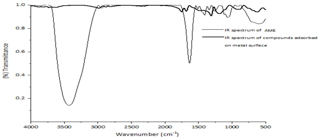
**Figure 8:** FT-IR Spectra of AME and compounds adsorbed on the mild steel surface.
