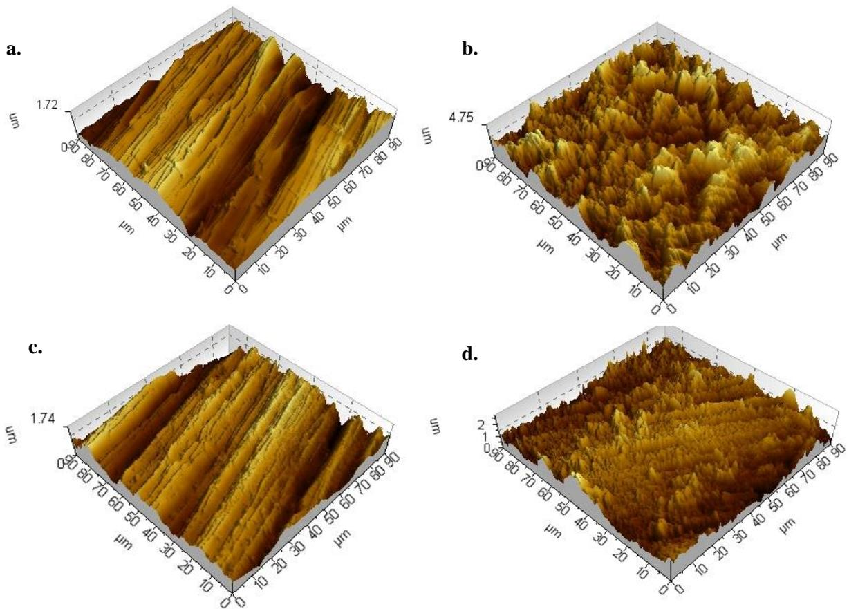
**Figure 7:** The 3D topographies of mild steel coupons obtained using AFM (a) before immersion (b) after immersion for 20 min at 25°C in Conc.HCl (c) AME (18 g/L) with Conc. HCl (d) Clarke solution
