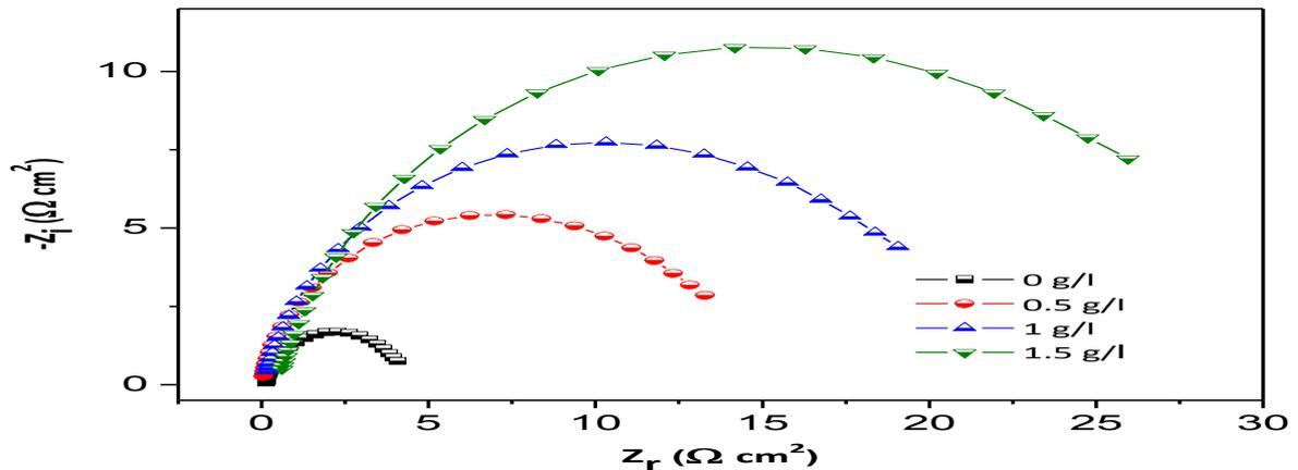
**Figure 4:** Nyquist plots for the corrosion of mild steel in 4 N HCl in the presence and absence of different concentrations of AME at 25°C
