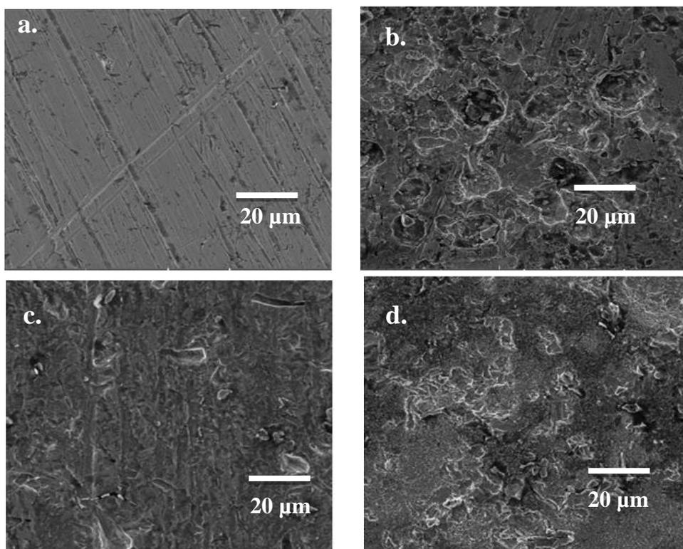
**Figure 6:** Micrographs of mild steel surface (a) before immersion (b) after immersion for 20 min at 25°C in Conc.HCl (c) AME (18 g/L) with Conc.HCl (d) Clarke solution
