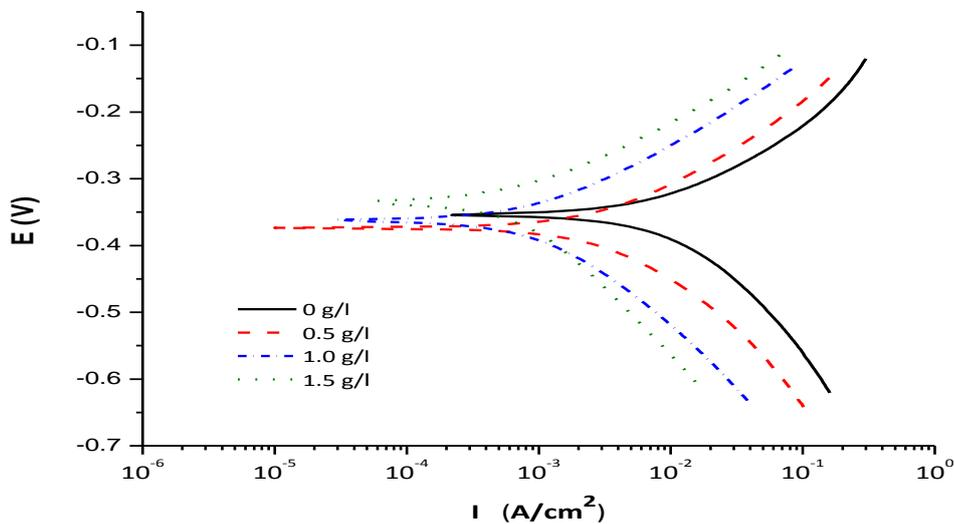
**Figure 3:** Potentiodynamic polarization curves for mild steel in 4 N HCl in the absence and presence of different concentrations of AME at 25°C
