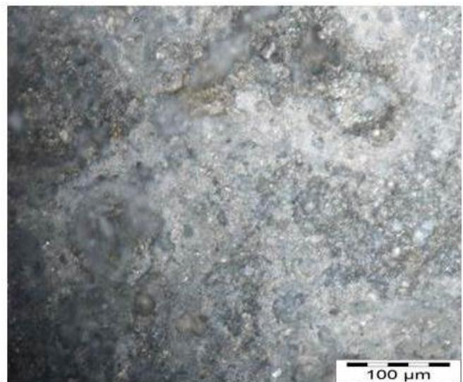
**Figure 4:** Morphology of Zn-40ZnO-1.0 A composite coating
