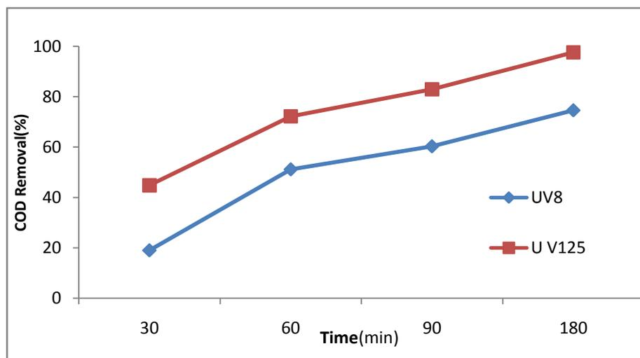
**Figure 3:** Effect of UV irradiation intensity and time on the removal COD
