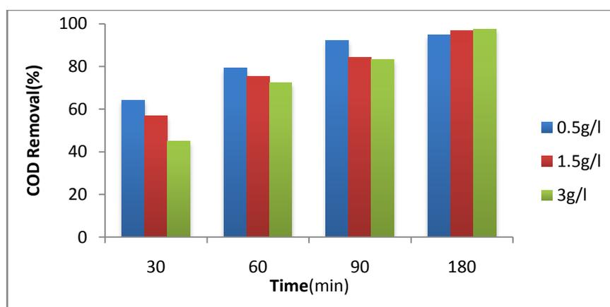
Figure 5: Effect of TiO<sub>2</sub> concentration on COD removal
