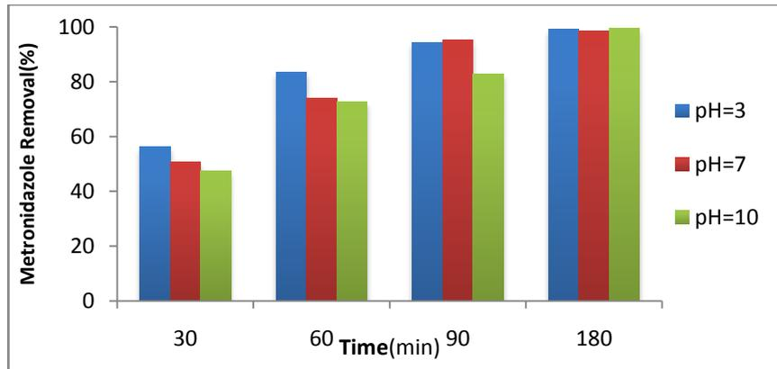
Figure 6: Effect of pH on the removal of metronidazole
