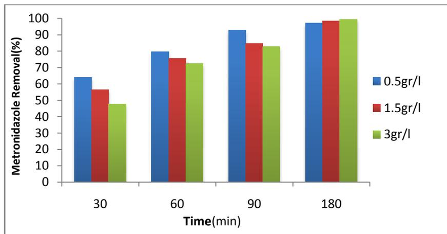
Figure 4: Effect of TiO<sub>2</sub> concentration on the removal efficiency of metronidazole
