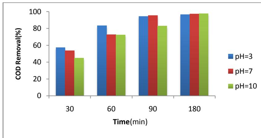
Figure 7: Effect of pH on COD removal
