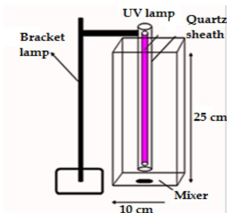
Figure 1: Photocatalytic reactor
