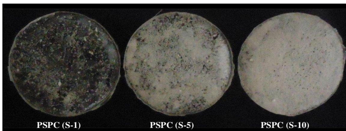
**Figure 1.** The photographs of the developed TiO<sub>2</sub>-strewn PS photocatalysts
