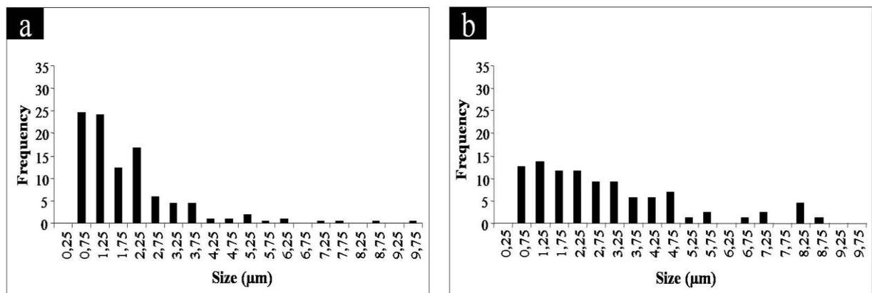
**Figure 7:** Grain size distribution of bainitic ferrite **a)** edge **b)** center.
