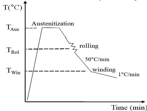
**Figure 1:** Thermomechanical treatments applied to M800HY steel.
