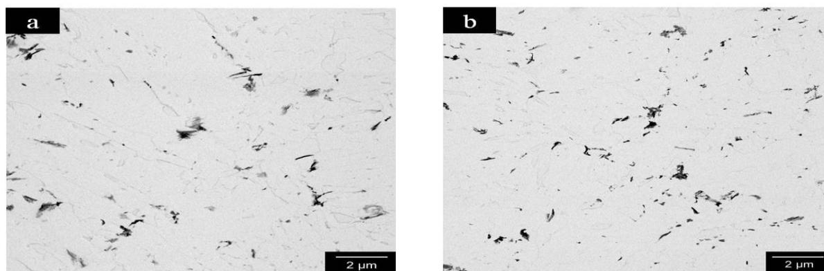
**Figure 3:** Transmission electron micrographs of replicas showing cementite particles **a)** edge **b)** center.
