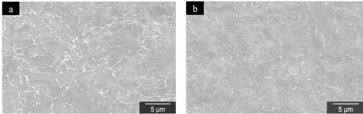
**Figure 5:** SEM micrographs showing the microstructures revealed by electrolytic etching **a)** edge **b)** center.
