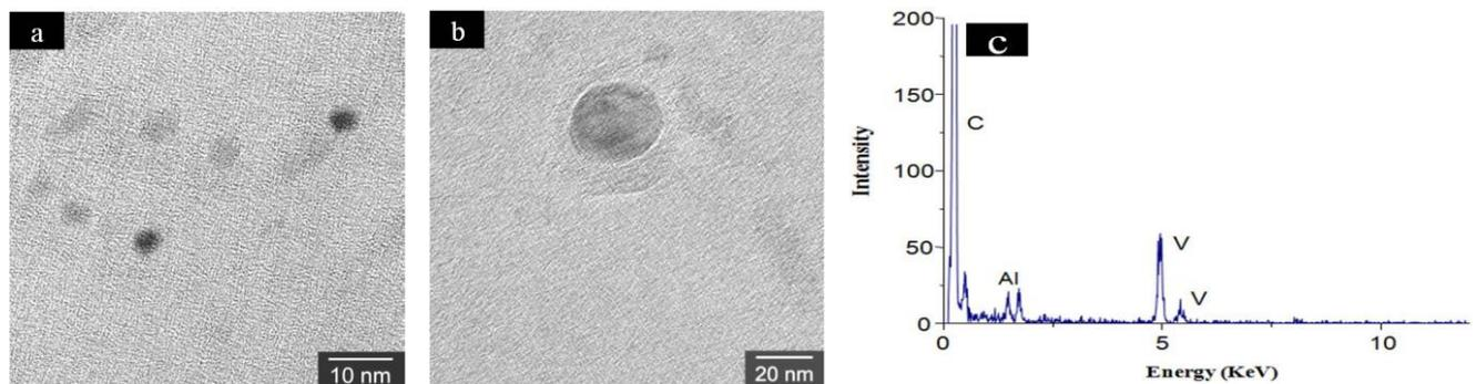
**Figure 4:** Transmission electron micrographs of replicas showing vanadium carbide particles
