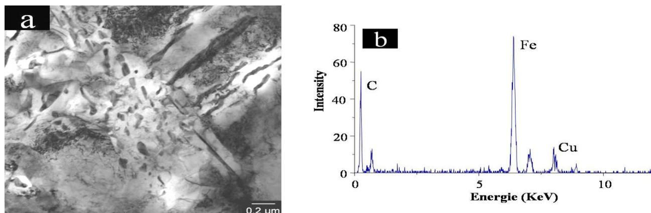
**Figure 2:** Transmission electron micrograph of thin section showing the type of cementite particles present in the different samples and EDS spectrum.
