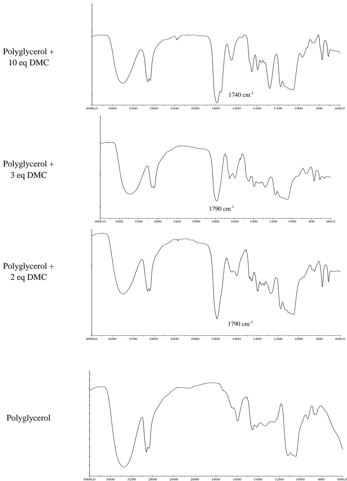
**Figure 2:** FTIR spectra of reaction product of PG3 with different amount of DMC
