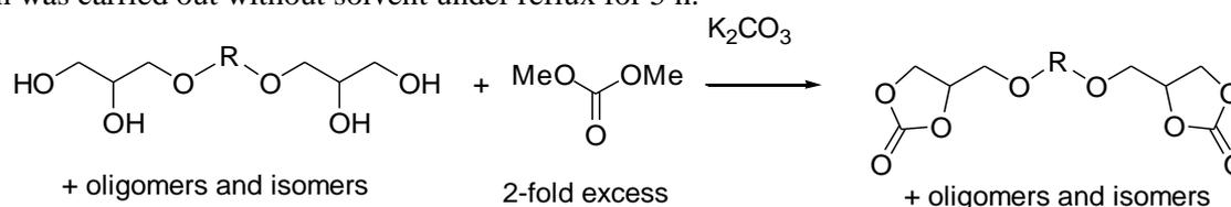
**Figure 1:** Reaction of PG3 mixture with DMC
