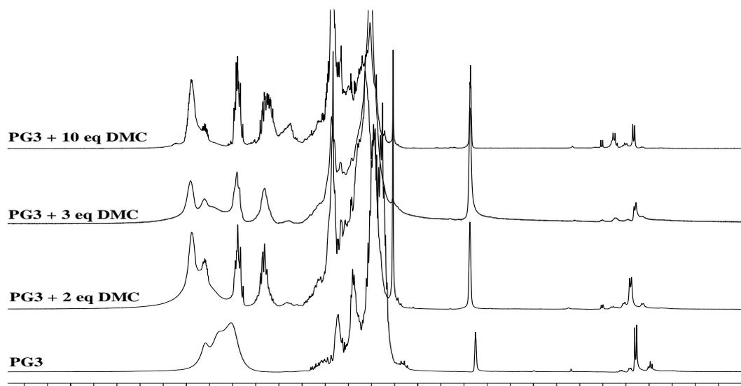
**Figure 3:**  $^1\text{H}$  NMR spectra of reaction product of PG3 with different amount of DMC (DMSO  $d_6$ , 400 MHz)
