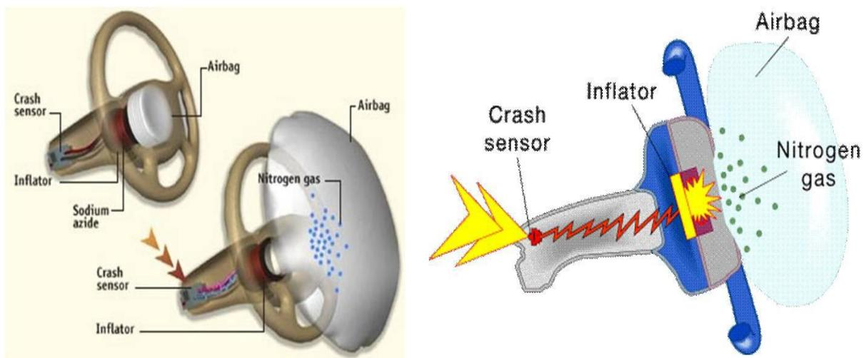
Figure 1: airbag structure and performance
