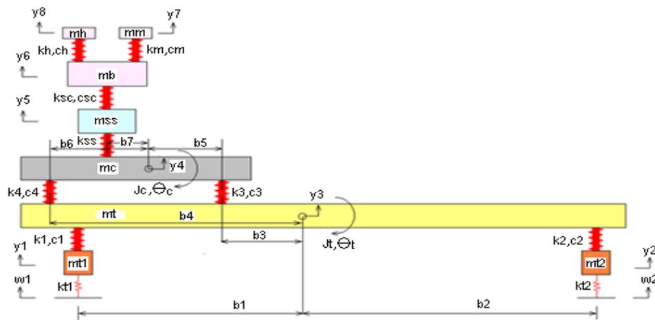
Figure 6: 10 dof vehicle vertical model
