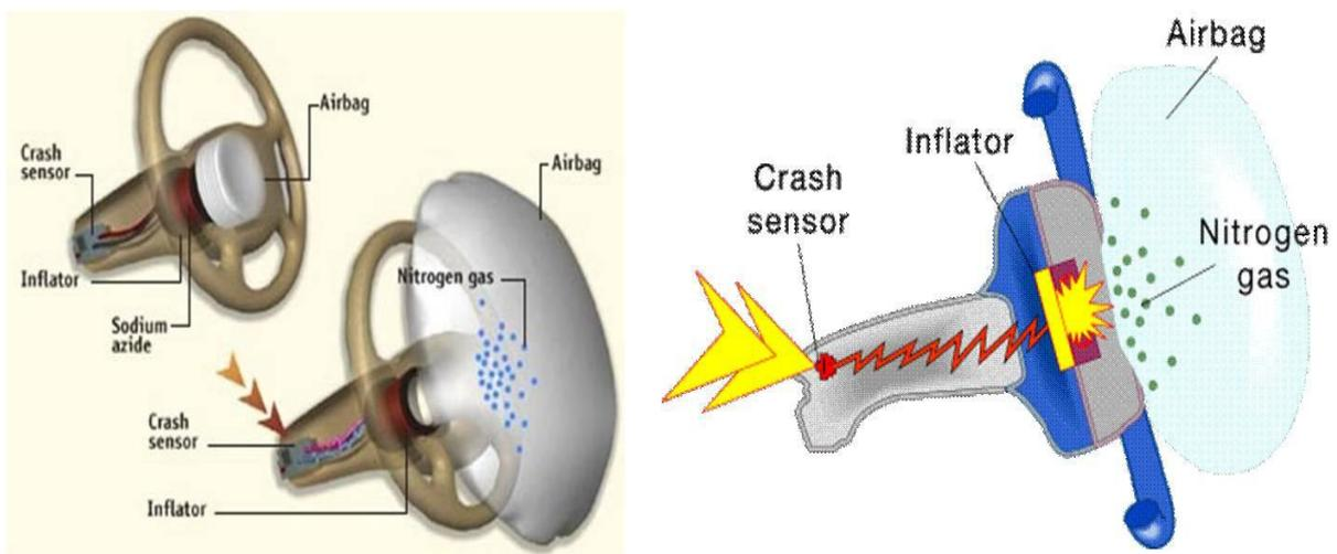
Figure 1: airbag structure and performance
