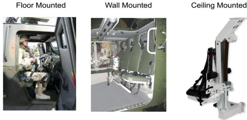
Figure 5: suspended seat connections
