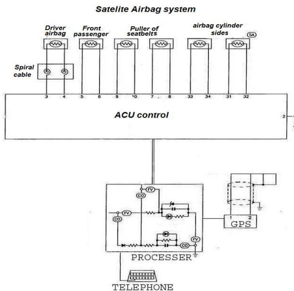
**Figure 3:** electrical circuit of smart air bag
