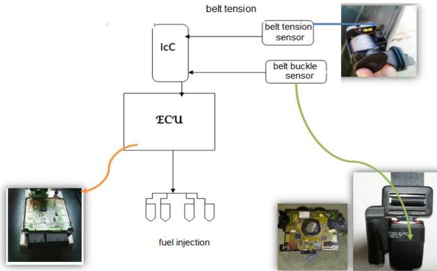
**Figure 8:** Smart seatbelt procedure
