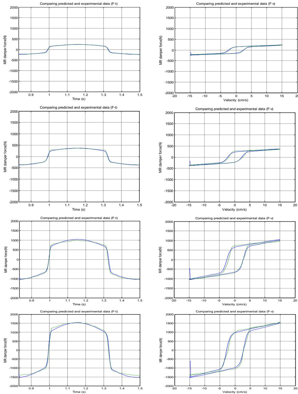
**Figure 15:** force-speed and force time graphs of MR damper - - - experimental \_\_\_\_\_ simulation model
