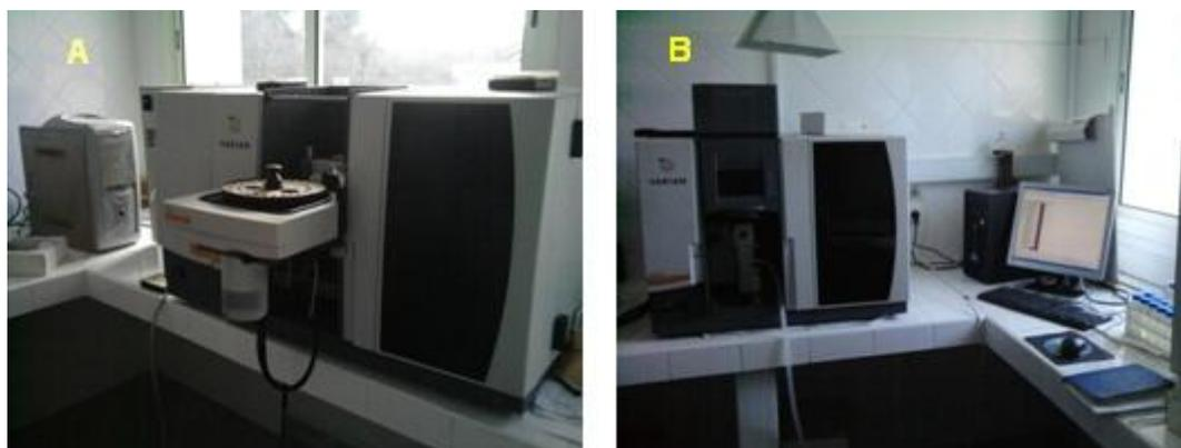
**Photo 2:** SAA (A: SAA with graphite and B: SAA with furnace)
