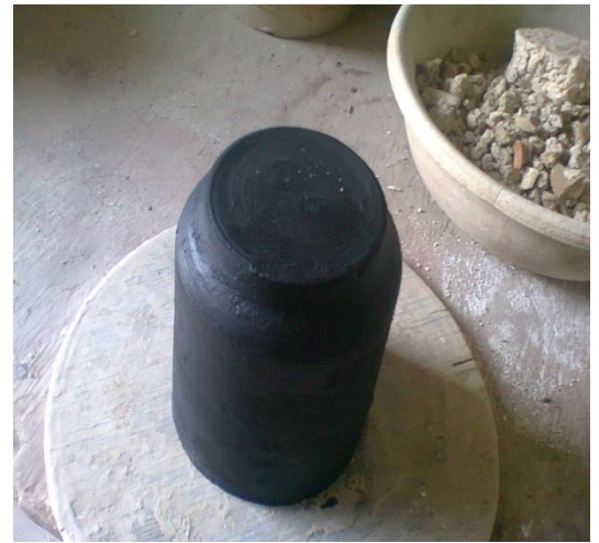
Figure 4: Crucible after been removed from the mould
