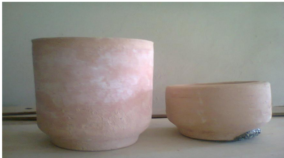
Figure 5: Glazed Crucible after been fired in the furnace
