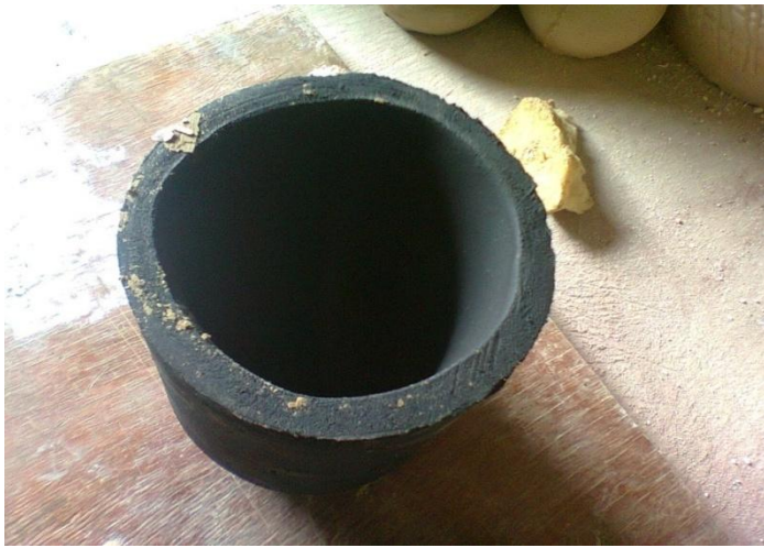
Figure 4: Crucible after been removed from the mould
