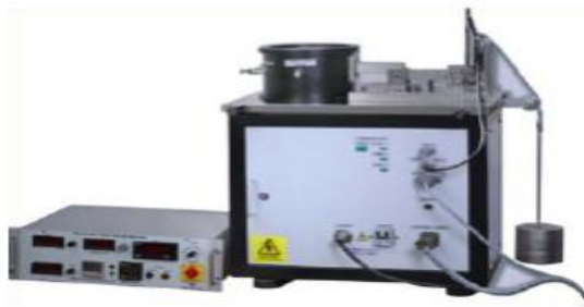
Figure 2 (a) : Pin on disc Wear Testing Machine
