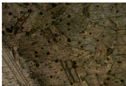
Figure 11: SEM micrograph of 304 stainless steel tested at 50°C, 100x.
