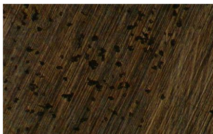
Figure 10: SEM micrograph of 304 stainless steel tested at 40°C, 100x.
