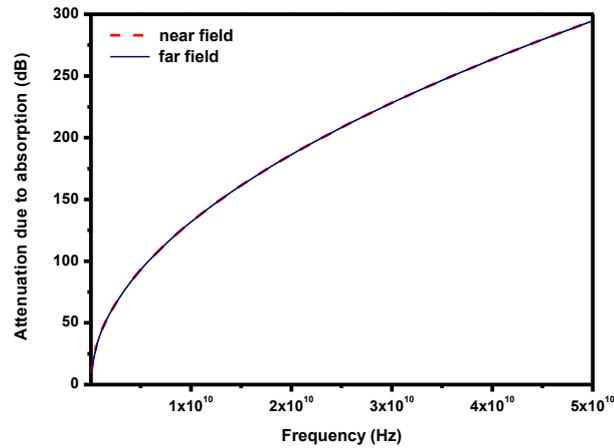
**Figure 3a:** Variation of attenuation due to the absorption as a function of frequency for (LDPE/V<sub>2</sub>O<sub>3</sub>) conducting polymer composite in near and far field.
