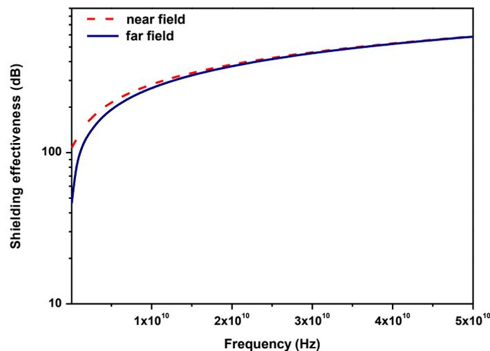
**Figure 2c:** Variation of electromagnetic shielding efficiency as a function of frequency for (HDPE/V<sub>2</sub>O<sub>3</sub>) conducting polymer composite in near and far field.
