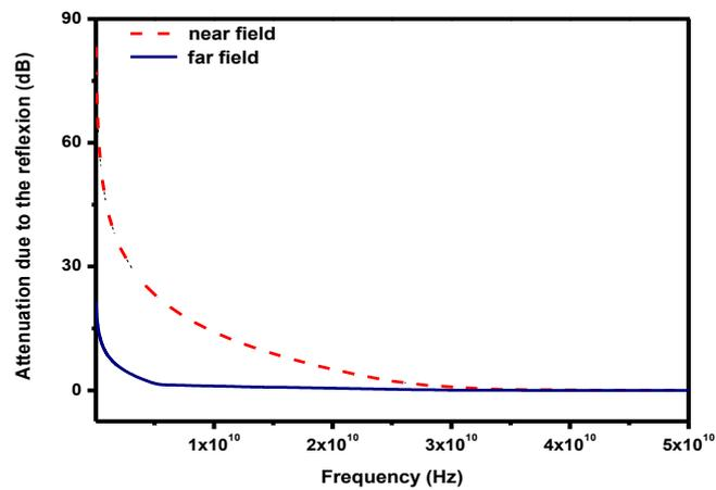
**Figure 3b:** Variation of attenuation due to the reflexion as a function of frequency for (LDPE/V<sub>2</sub>O<sub>3</sub>) conducting polymer composite in near and far field.
