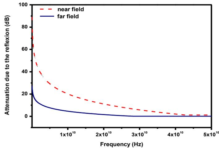
**Figure 2b:** Variation of attenuation due to the reflexion as a function of frequency for (HDPE/V<sub>2</sub>O<sub>3</sub>) conducting polymer composite in near and far field
