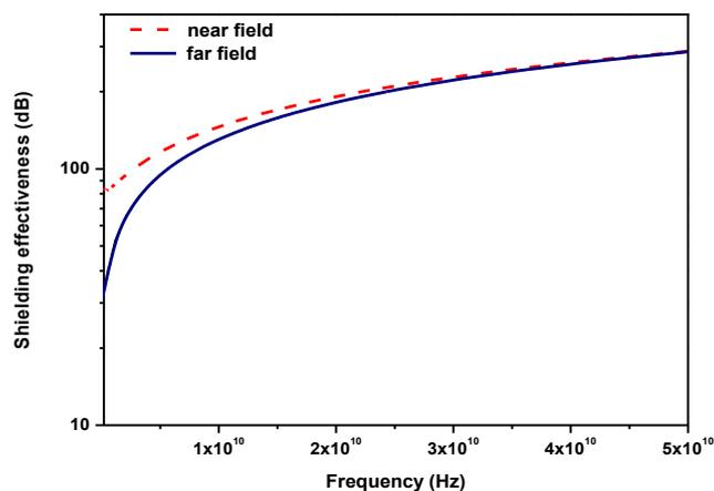
**Figure 3c:** Variation of electromagnetic shielding efficiency as a function of frequency for (LDPE/V<sub>2</sub>O<sub>3</sub>) conducting polymer composite in near and far field.
