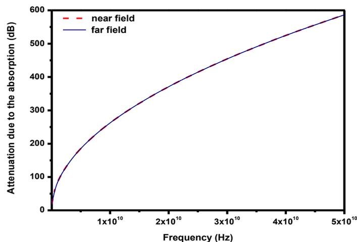
**Figure 2a:** Variation of attenuation due to the absorption as a function of frequency for (HDPE/V<sub>2</sub>O<sub>3</sub>) conducting polymer composite in near and far field.
