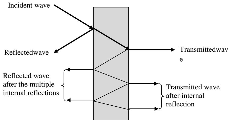
**Figure1:** Schematic showing electromagnetic shielding.
