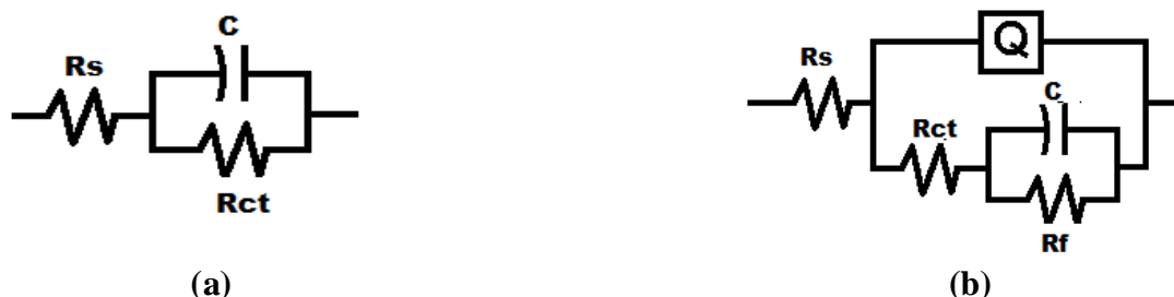
Figure 3: Equivalent circuit used to fit the experimental EIS data for the corrosion of welded maraging steel specimen in 1.0 M sulphuric acid at 30 °C (a) for the blank solution and (b) in the presence of inhibitor.
