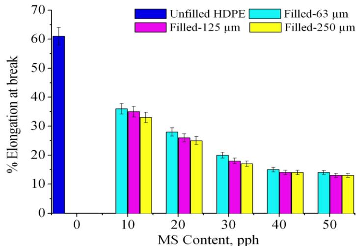
**Figure 4:** % Elongation at break graph for MS/HDPE composites
