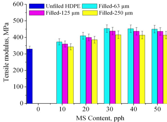
**Figure 3:** Tensile modulus graph for MS/HDPE composites
