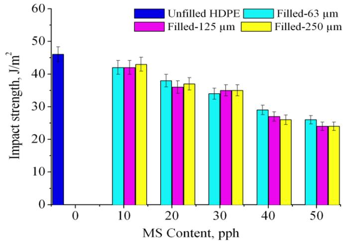
Figure 6: Impact strength graph for MS/HDPE composites
