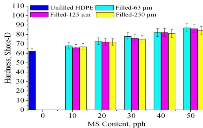
Figure 7: Hardness graph for MS/HDPE composites
