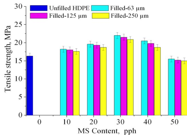
**Figure 2:** Tensile strength graph for MS/HDPE composites
