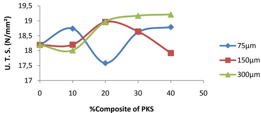
**Figure 4:** Plot of U. T. S. against %composition of PKS.
