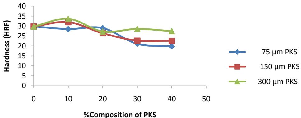
**Figure 5:** Plot of hardness against % composition of PKS.
