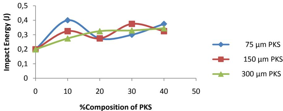
**Figure6:** Plot of impact energy against %composition of PKS.
