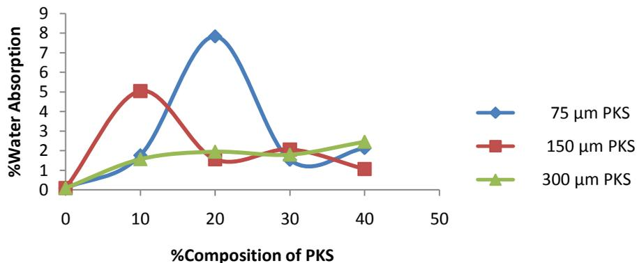
**Figure 2:** Plot of water absorption against %composition of PKS
