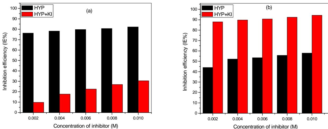
**Figure 7:** Synergistic effect of iodide ions on the inhibition efficiency of HYP on the corrosion of (a) aluminium and (b) mild steel in 0.1 M H<sub>2</sub>SO<sub>4</sub> at 303 K.
