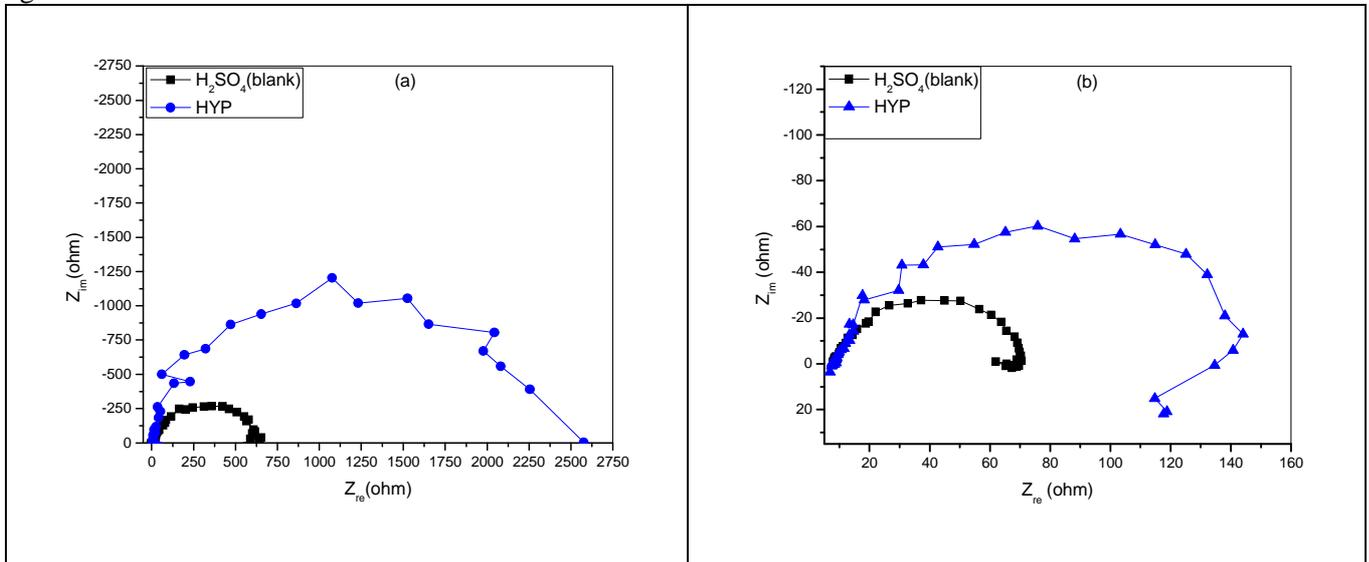
**Figure 3:** Impedance spectra for (a) aluminium and (b) mild steel in 0.1 M  $H_2SO_4$  in the absence and presence of 0.01 M hypoxanthine (HYP) at 303 K.
