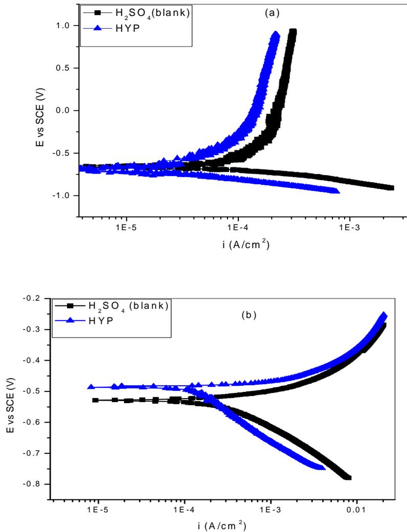
**Figure 4:** Polarisation curves for (a) aluminium and (b) mild steel in 0.1 M H<sub>2</sub>SO<sub>4</sub> in the absence and presence of 0.01 M hypoxanthine (HYP) at 303 K.
