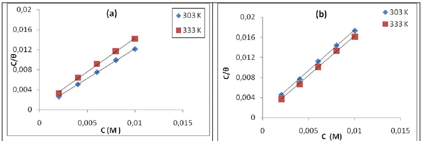
**Figure 5:** Langmuir isotherm for the adsorption of hypoxanthine (HYP) onto (a) aluminium (b) mild steel surface in 0.1 M H<sub>2</sub>SO<sub>4</sub> at 303 and 333 K respectively.
