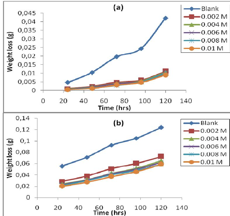
**Figure 2:** Variation of weight loss (g) with time (hrs) for the corrosion of (a). aluminium and (b). mild steel in 0.1 M H<sub>2</sub>SO<sub>4</sub> containing various concentrations of hypoxanthine (HYP) at 303 K.
