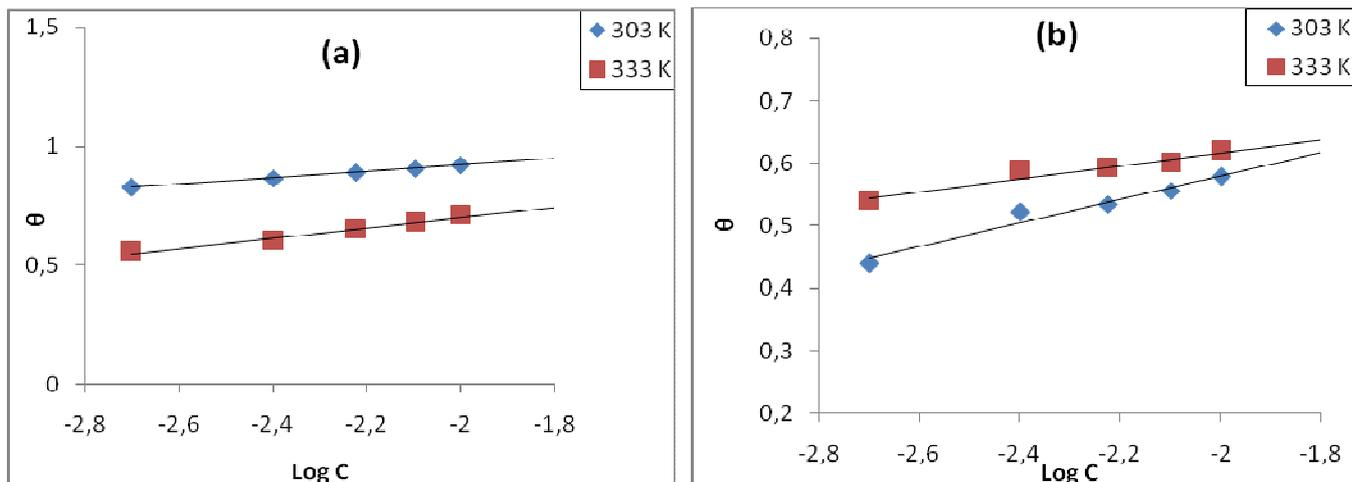
**Figure 6.** Temkin isotherm for the adsorption of hypoxanthine (HYP) onto (a) aluminium (b) mild steel surface in 0.1 M  $H_2SO_4$  at 303 and 333 K respectively.
