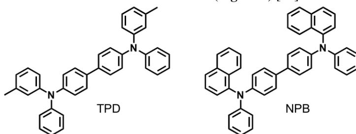
Figure 5 : Commonly used components in holes transport layer. TPD =N,N-diphenyl-N,N-bis(3-methylphenyl)-1,1-biphenyl-4,4-diamine; NPB = 1,4-bis(1-naphthylphenylamino)biphenyl
