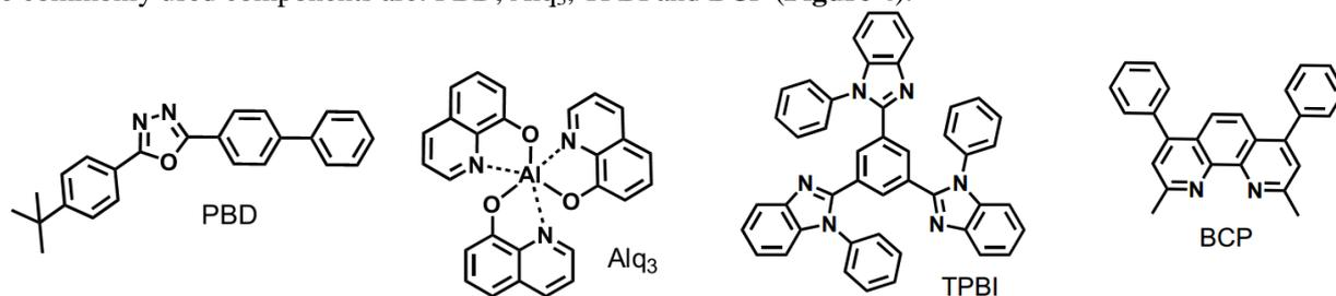
Figure 4 : Commonly used components in electrons transport layer.
