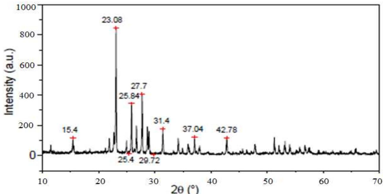
Fig. 3. XRD pattern of the sulfur nanoparticles [12].
