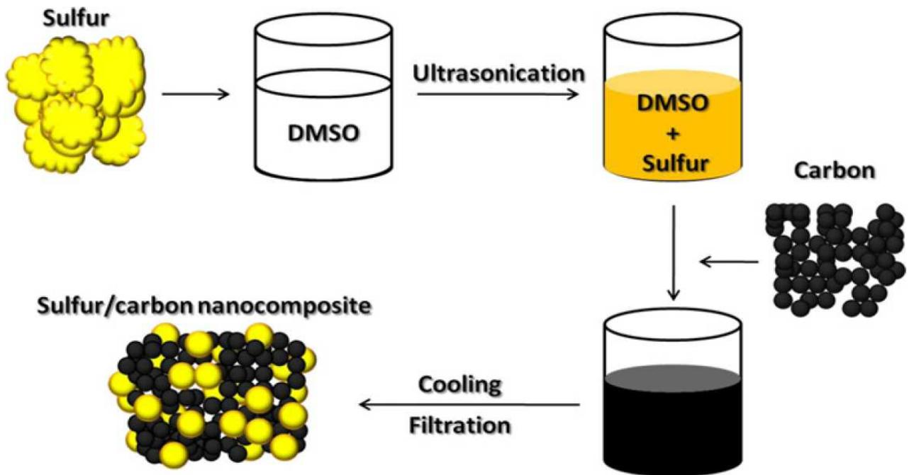
Fig. 1. Schematic of the solution processing for the preparation of sulfur/carbon [27]
