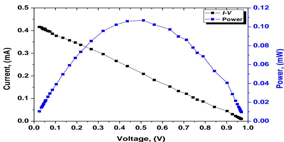
**Figure 3** The load current-voltage characteristics and power versus voltage of zinc/Rh.B aqueous solution/carbon dye electrochemical cell.
