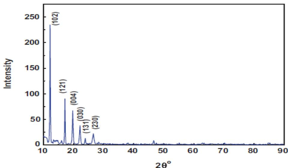
**Figure 2** X-ray diffraction pattern of Rh.B in powder form [11].
