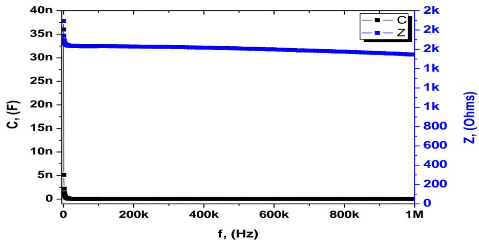
**Figure 7** Capacitance and impedance as a function of the applied frequency of zinc/Rh.B aqueous solution/carbon dye electrochemical cell.
