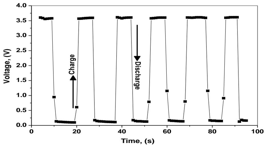
**Figure 6** Life cycles of charge/discharge of the voltage-time of zinc/Rh.B aqueous solution/carbon dye electrochemical cell.
