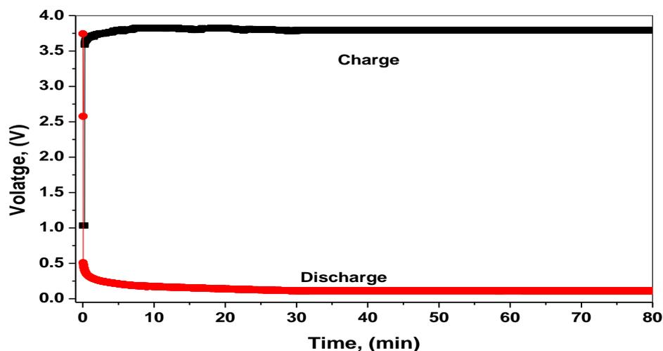
**Figure 4** Charge/discharge of the voltage-time of zinc/Rh.B aqueous solution/carbon dye electrochemical cell.
