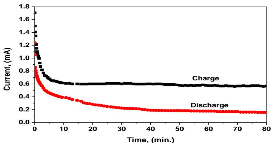
**Figure 5** Charge/discharge of the current-time of zinc/Rh.B aqueous solution/carbon dye electrochemical cell.
