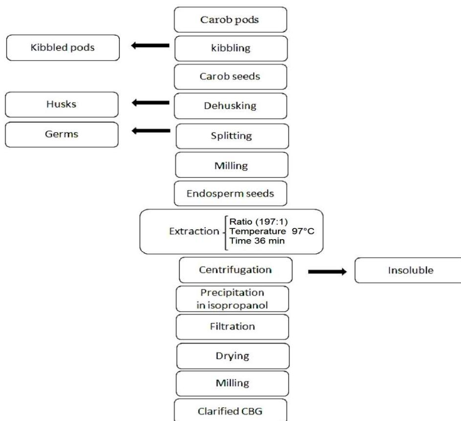
**Figure 2.** Extraction and purification process of carob been gum.
