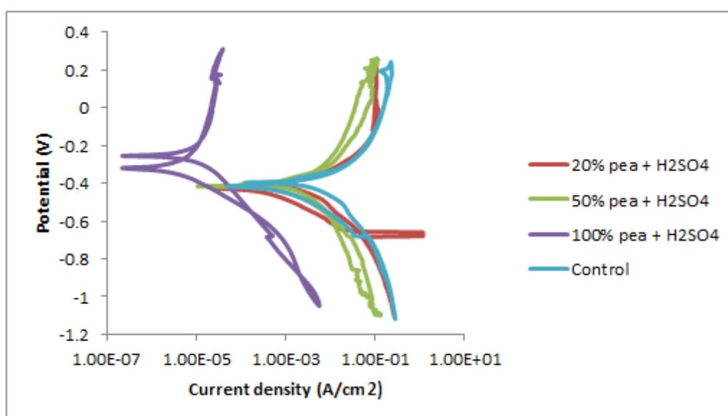
**Figure 2:** Linear polarization of mild steel in 2M H<sub>2</sub>SO<sub>4</sub> solution/*Arachis hypogaeae* environment at 298K
