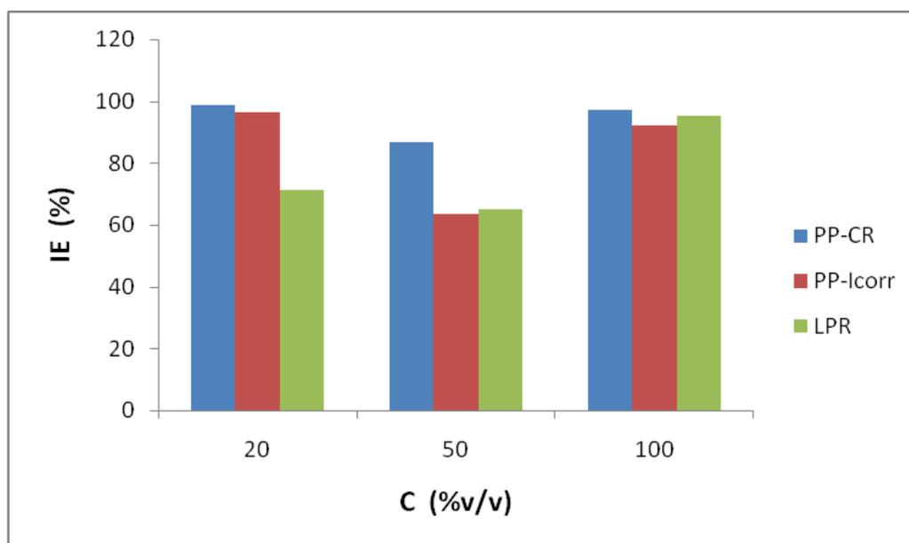
**Figure 5:** Comparative chart of inhibitor efficiency (IE) for 2M  $H_2SO_4$  solution/*Arachis hypogaeae* concentration obtained from potentiodynamic polarization-corrosion rate (PP-CR), potentiodynamic polarization-corrosion current (PP-Icorr) and linear polarization resistance (LPR)
