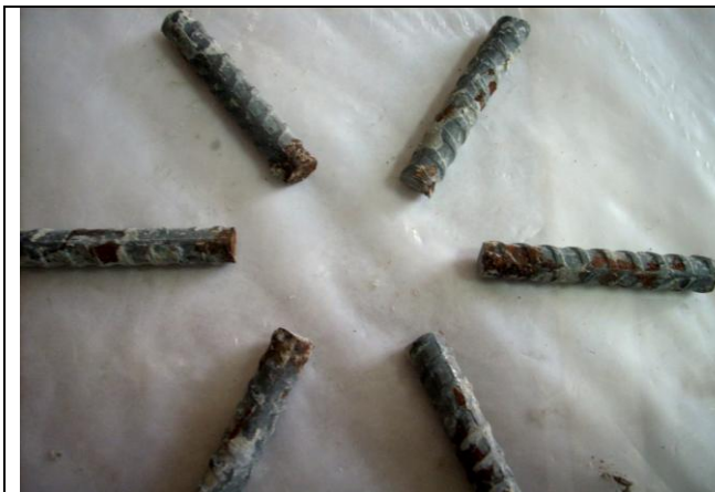
Fig. 1.1: Corrosion of steel bar embedded in blank sample after 90 days of exposure.
