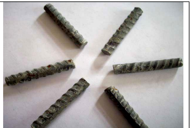
Fig. 1.2: Corrosion of steel bar embedded in concrete with 3% calcium palmitate and 1.5% calcium nitrite after 90 days of exposure.
