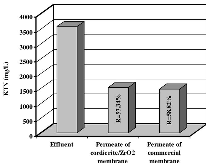
Fig. 10. Reduction of KTN content by microfiltration process.
