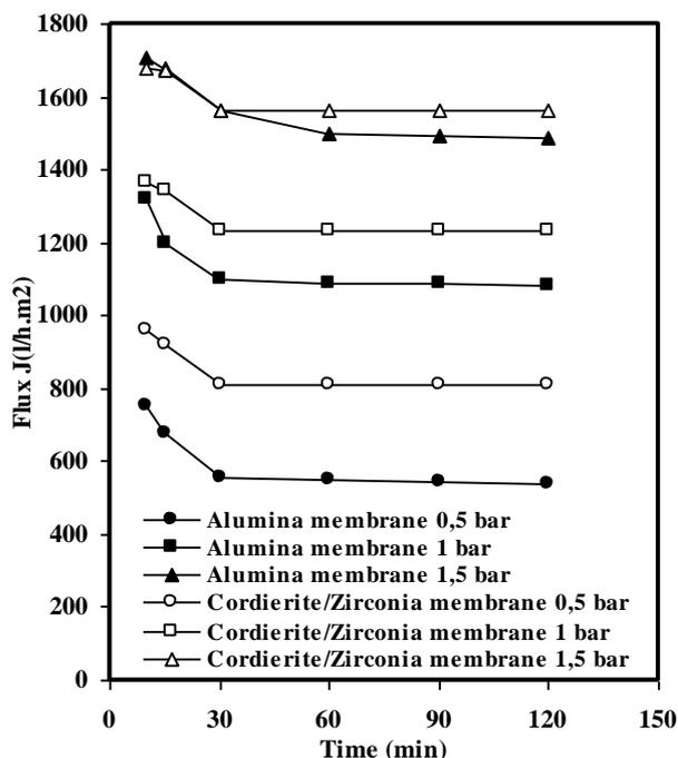
Fig. 4. Water flux vs. operating time.
