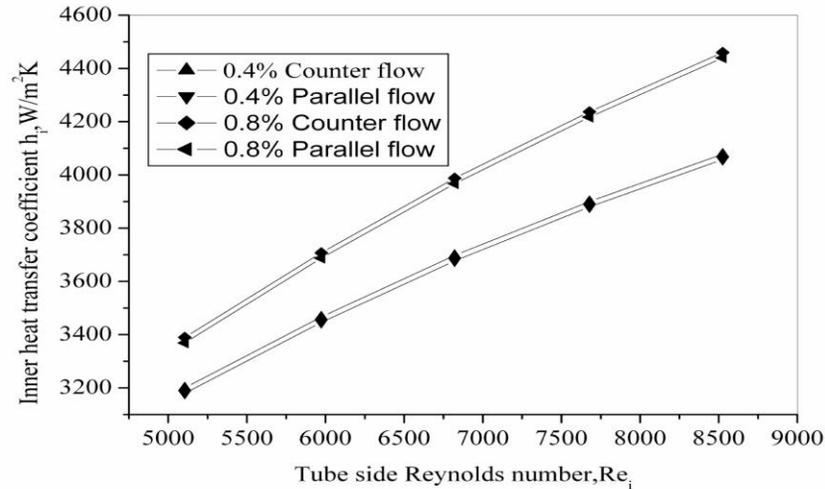
**Figure 6:** Variation of inner heat transfer coefficient with tube side Reynolds number
