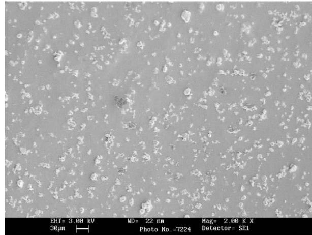
Figure 2: SEM image of Al<sub>2</sub>O<sub>3</sub> nanoparticles
