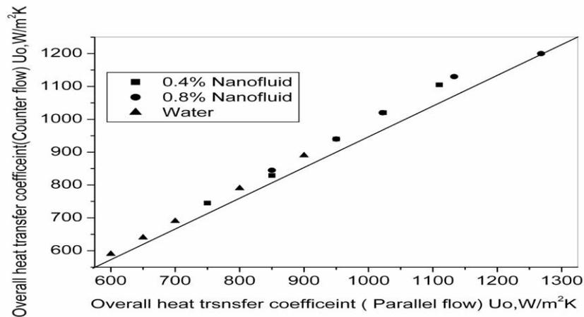
**Figure 5:** Comparison of overall heat transfer coefficient of counter and parallel flow configuration under laminar flow
