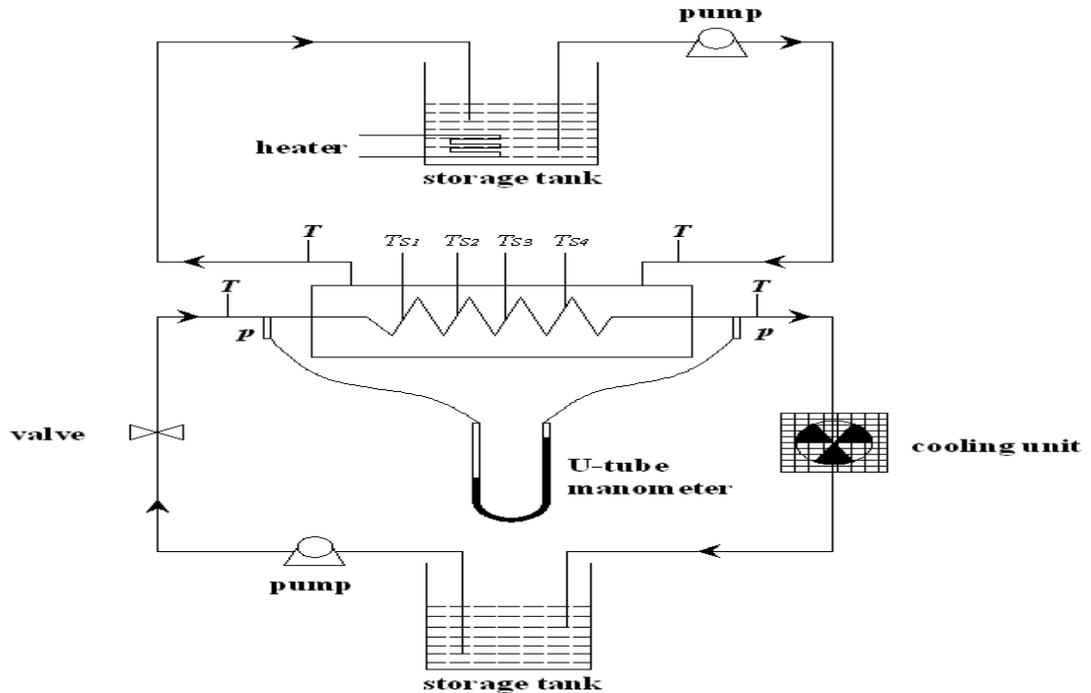
Figure 3: Flow diagram of experimental setup
