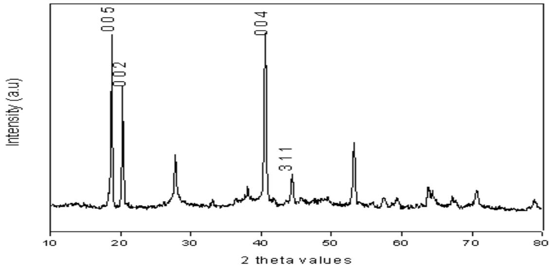
**Figure.1:** XRD pattern of  $\text{Al}_2\text{O}_3$  nanoparticles
