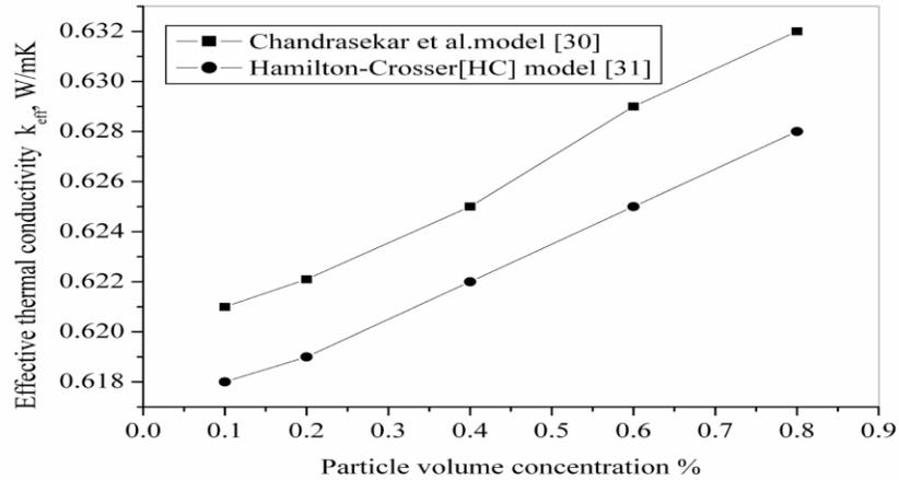
**Figure 4:** Thermal conductivity of Al<sub>2</sub>O<sub>3</sub> / water nanofluid as a function of particle volume concentration
