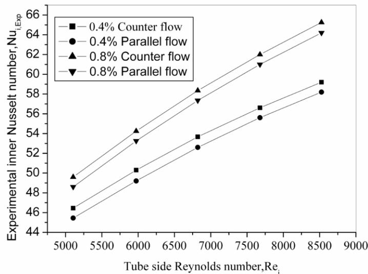
**Figure 7:** Variation of experimental inner Nusselt number with tube side Reynolds number
