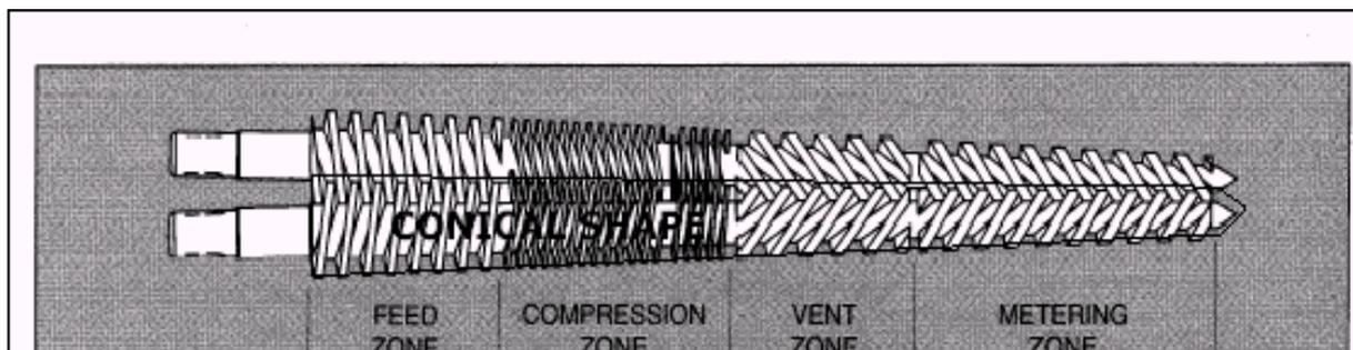
**Fig. 1.** Conical twin screw extruder
