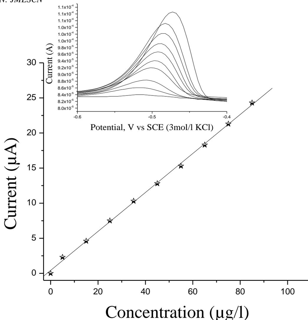
**Figure 1:** Calibration curves for lead in 0.1M acetate buffer (pH 4.5) containing 500 µg.L<sup>-1</sup> of bismuth. Lead was ranged from 5 to 85µg.L<sup>-1</sup>.
