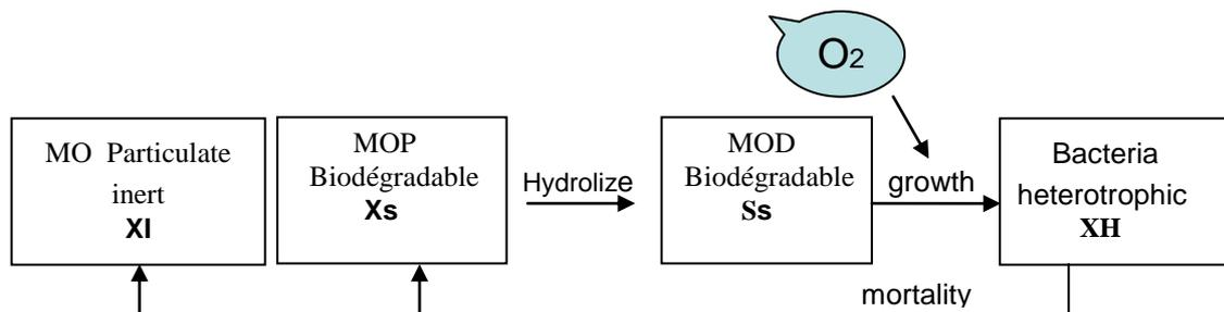
**Figure 1:** Concept describing the biological breakdown of the dissolved and Particulate organic matter in ASM1 (IWA; 1987)
