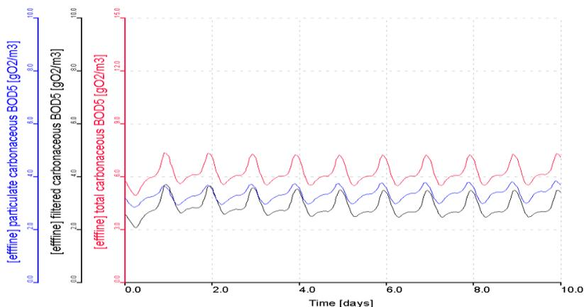
**Figure 3:** DBO5 and its fractions at exit of clarifier
