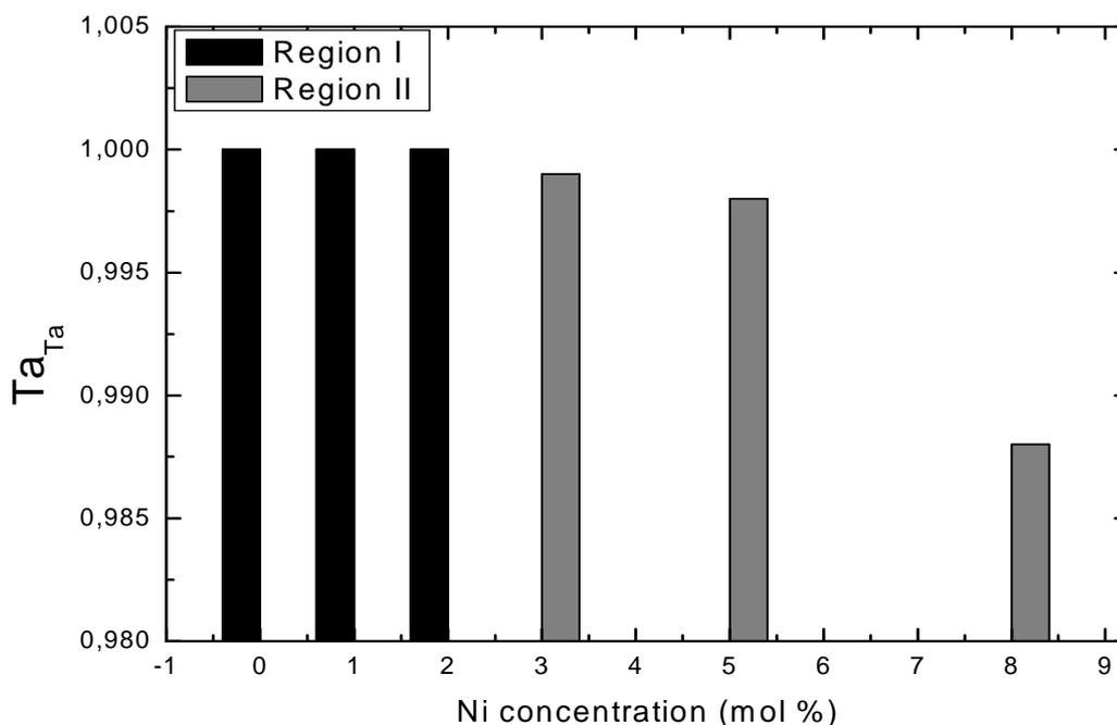
**Figure 1:** Plot of normal Ta site ( $Ta_{Ta}$ ) as function of Ni doping concentration.
